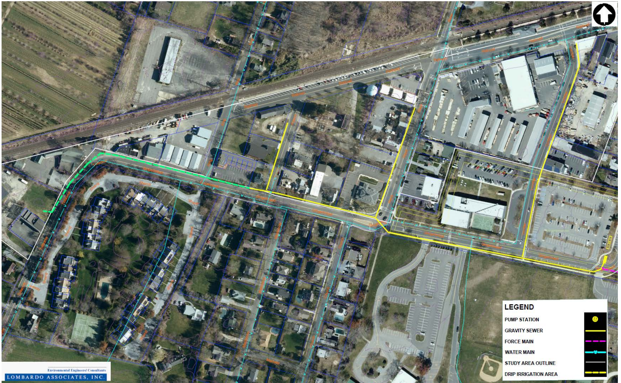
Figure E-3 Gingerbread Lane Sewer Layout
