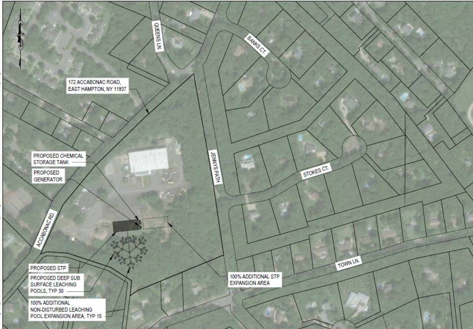
1 172 Accabonac Road BESST and SBR Conceptual Layout SCALE: 1" = 200' - 0"
