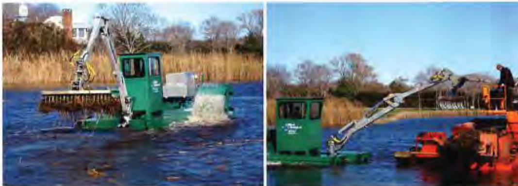
LITTLE HOOK POND - HYDRO-RAKE WITH FULL LOAD OF PHRAGMITES ROOTS AND RHIZOMES (LEFT); AND THEN TRANSFERRING DUG MATERIAL TO TRANSPORTER (RIGHT). 12/2006
