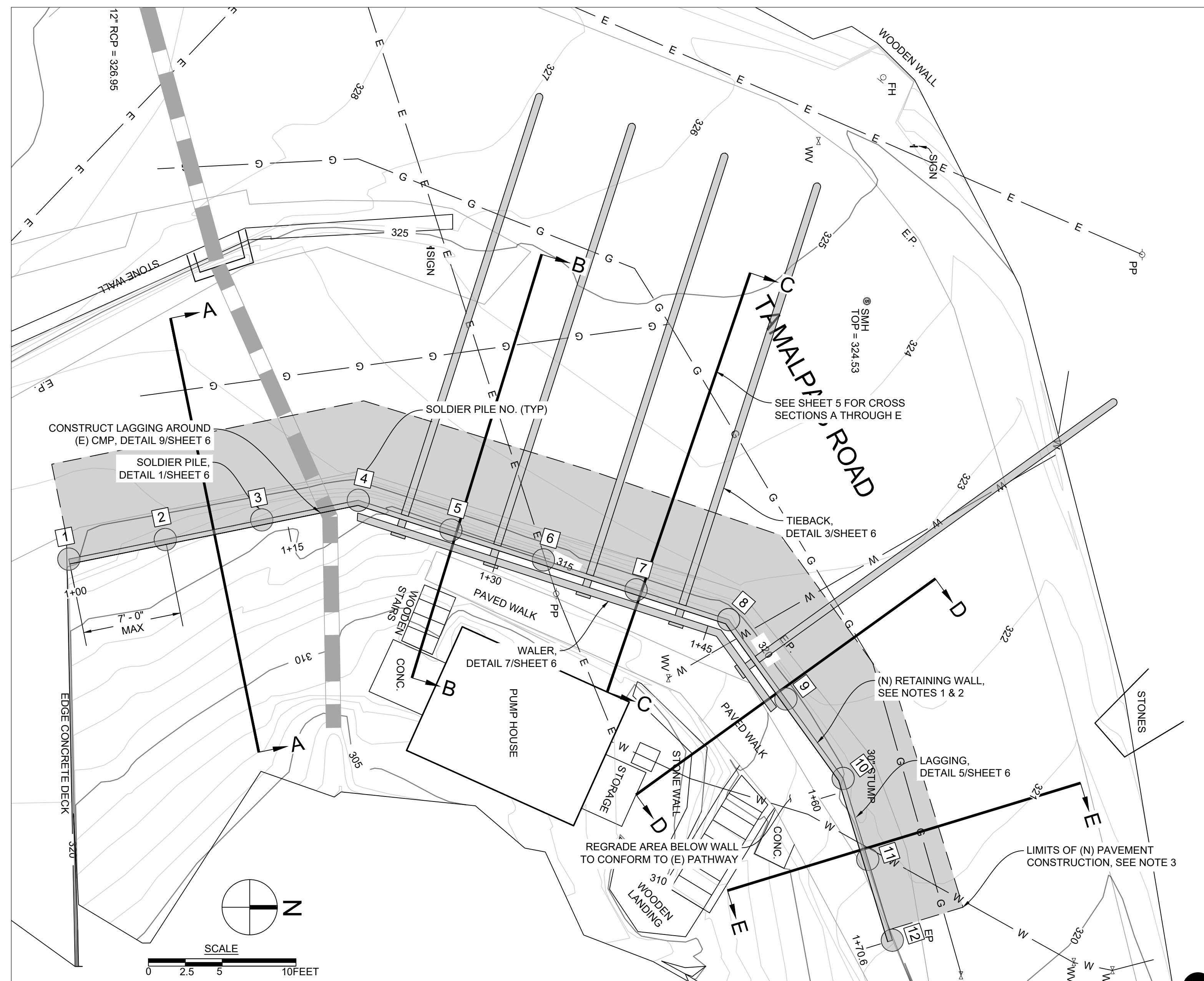
RETAINING WALL PLAN (SCALE: 1" = 5'-0")
