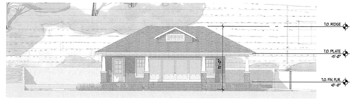
1 A.D.U. ELEVATIONS - SOUTH A3.2 1/8" = 1'-0"
