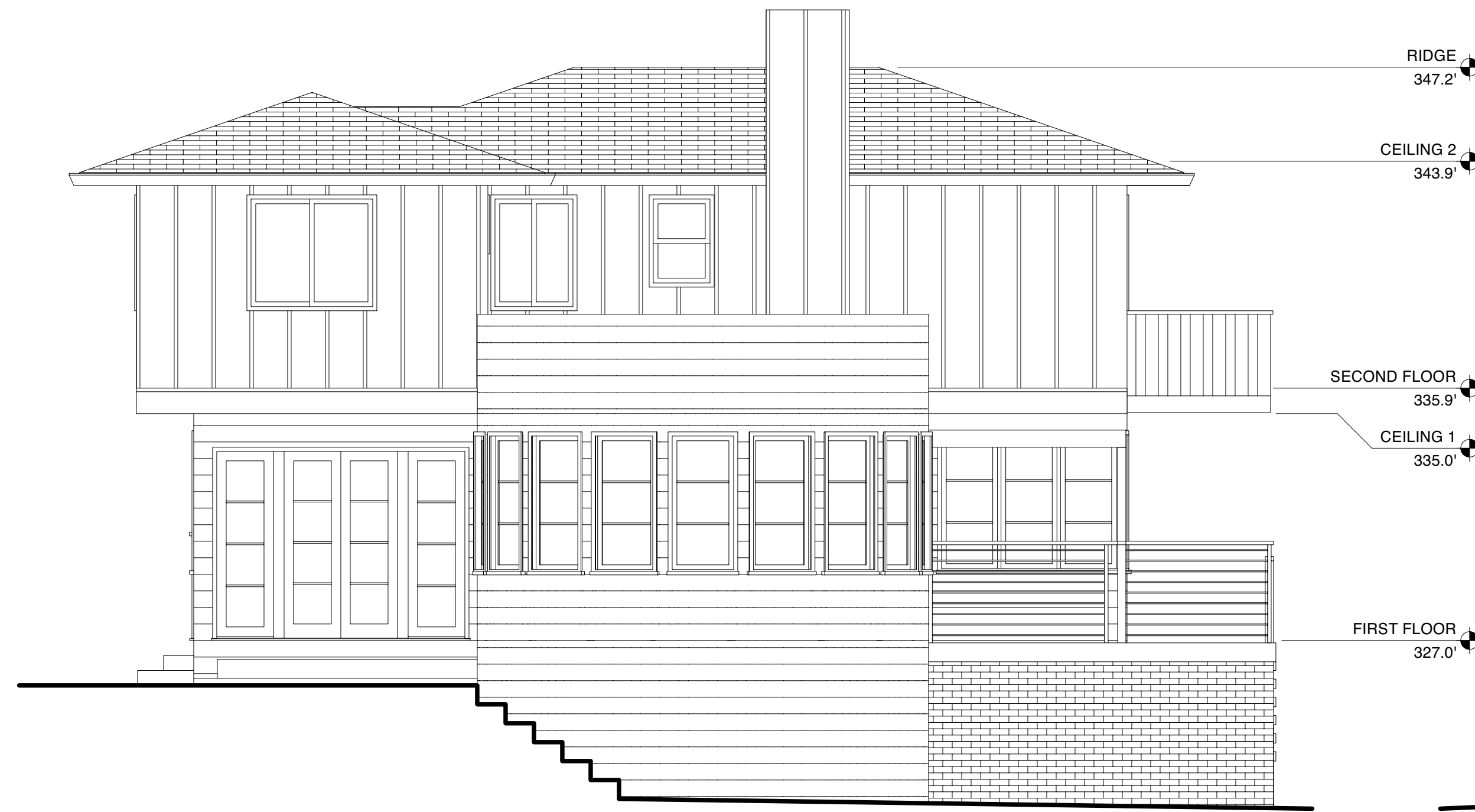
1 REAR (SOUTH) ELEVATION - EXISTING Scale: 1/4" = 1'-0"
