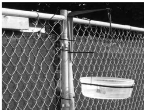
Photo 2. Dust fall sampler apparatus. Source: University of Illinois at Chicago
