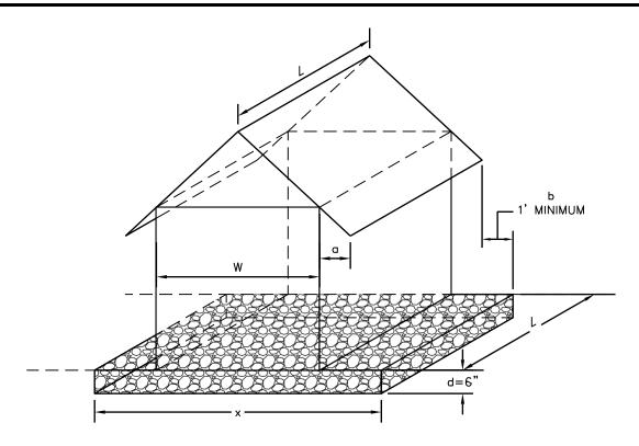
$\overline{L}$  = LENGTH OF STRUCTURE = LENGTH OF SEEPAGE BED (FT.)
