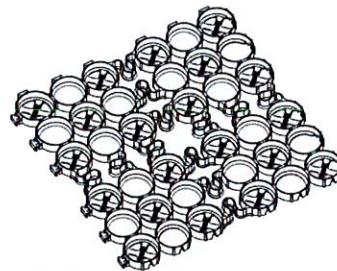
TRUEGRID BLOCK REFERENCE VIEW PREASSEMBLED & DELIVERED IN 4' x 4' SHEET. RECONFIGURED AS NEEDED. NO EXTRA TOOLING OR ACCESSORIES REQUIRED.
