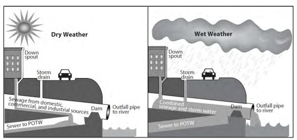
Figure 3-2: How a combined sewage and stormwater system handles wet weather U.S. Environmental Protection Agency (EPA)
