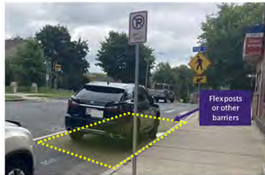
Flex posts could be used in instances like the situation pictured above to deter illegal parking and improve pedestrian visibility at the crosswalk
