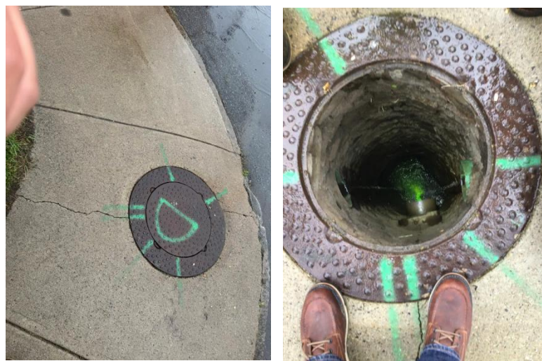
Figure 2-2: Dye Test Discharge in Storm Drain
