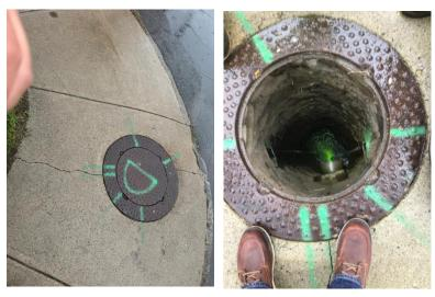
Figure 2-2: Dye Test Discharge in Storm Drain
