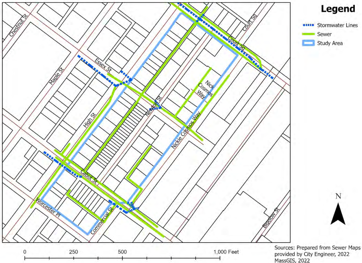
High-Appleton Study - Map 20: Study Area Sanitary Sewer and Stormwater Lines
