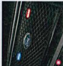
Grille LED lights , includes (2) buckle latching function and (2) LED side marker lights (driver side red, passenger side blue).
