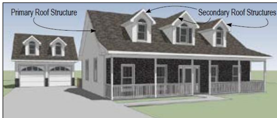
1149.03.16.I Figure 49.19 – Primary & Secondary Roof Structures
