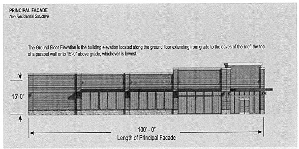
The Principal Facade shown above is in compliance with the Minimum Transparency requirements. The Principal Facade is 100' in length. The extended parapet wall is higher than 15'-0" so the 15'-0" maximum is utilized. The Ground Floor Elevation is 100' x 15'-0" = 1,500 sq feet. The windows upon this facade total 678 sq feet or 45.2%, thus meeting the 30% minimum standard.
