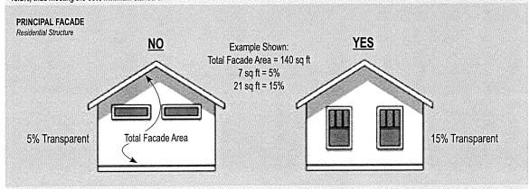
The Principal Facade shown above at left is not in compliance with the Minimum Transparency requirements. It is only 5% transparent based on the calculation. The Principal Facade shown above at right is in compliance with the Minimum Transparency requirements. It measures at 15% transparent.
