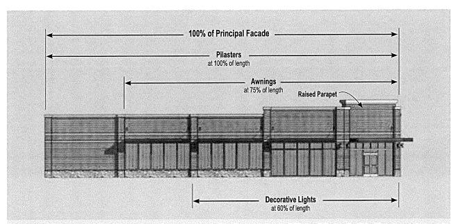
This Principal Facade is compliant with the Minimum Design Elements requirements. It has four design elements: 1) Pilasters, 2) Awnings, 3) a Raised Parapet over a Customer Entrance, and 4) Decorative Light Luminaires. The pilasters, awnings and decorative lights are applied along at least 50% of the facade's horizontal length.
