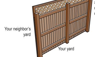
Note: The posts and structural supports must be on the inside of the fence.
