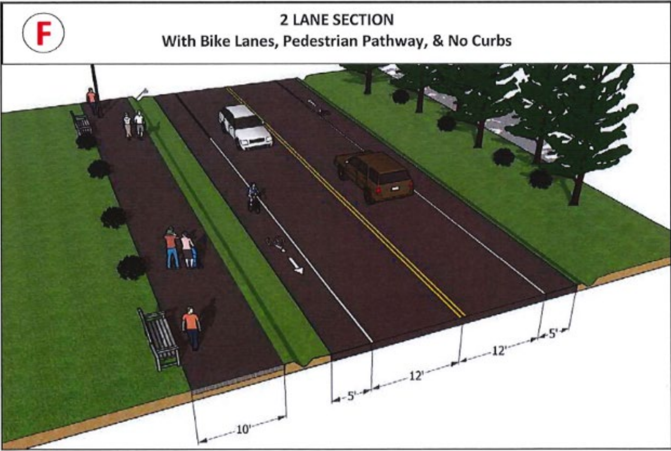
Figure 2-17: Roadway Cross-Sections (F)
