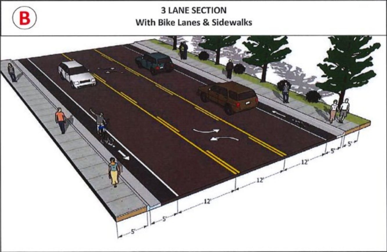
Figure 2-13: Roadway Cross-Sections (B)
