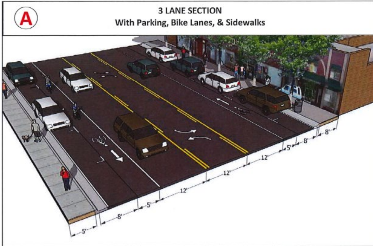
Figure 2-12: Roadway Cross-Sections (A)
