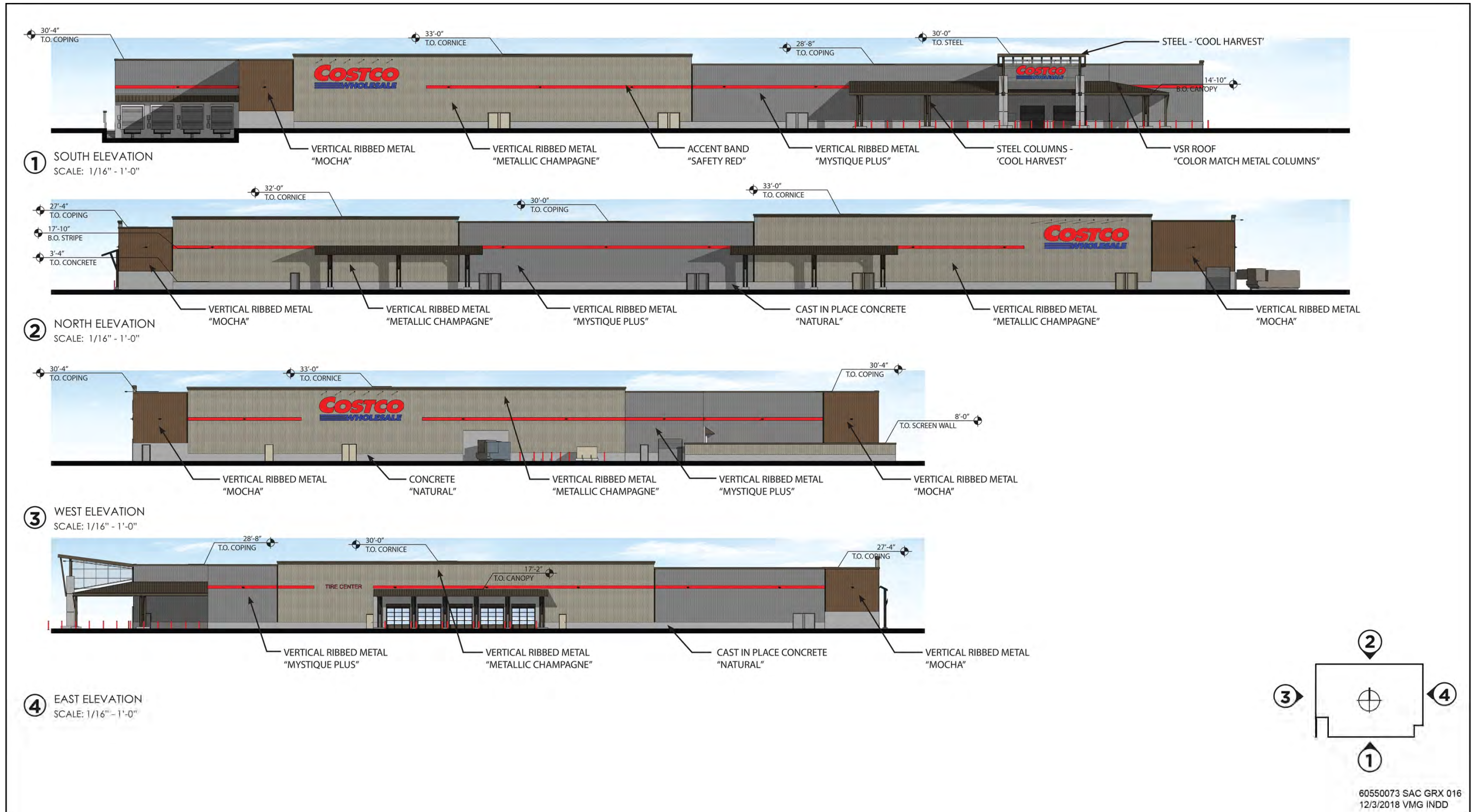
Figure 2-6. Warehouse Building Elevations
