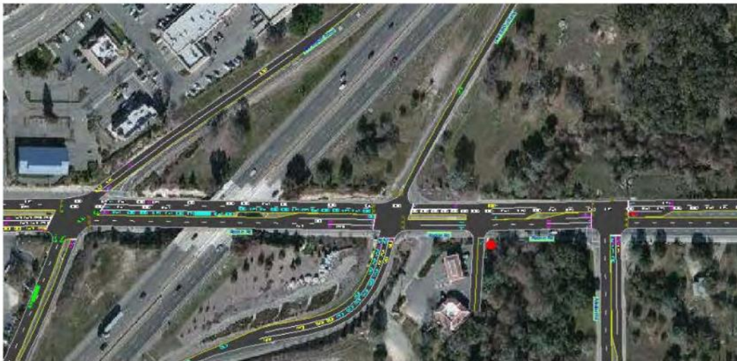
Image shows queue spillback (vehicles in blue) from the I-80 WB on-ramp, which adversely affects the EB ramps and Aguilar Road intersections.
