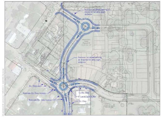
The roundabout conceptual layouts are based on the NCHRP Report 672, Roundabouts: An Informational Guide Second
