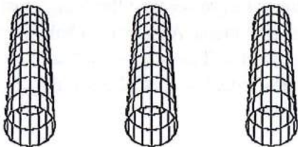
Cylinder vibrations of the barrel of an aluminum bat
