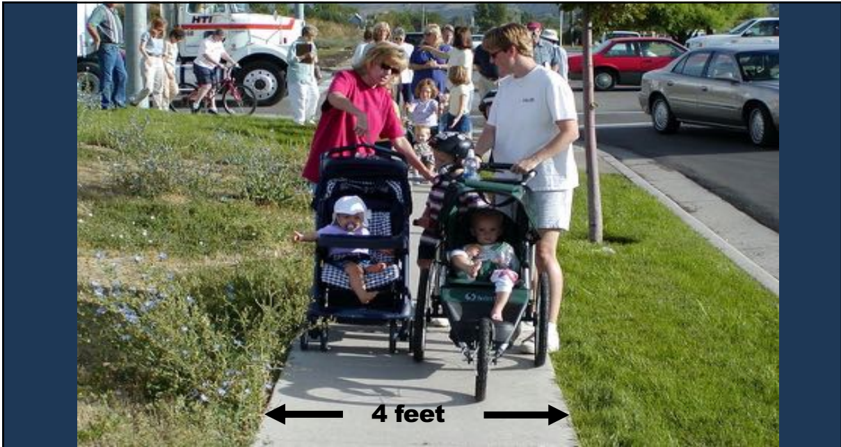
For two moms (or dads) with strollers, sidewalks need to be at least 5 feet wide
