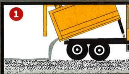
Spread additional material or additive (crushed rock, cement, fly ash, lime, etc.).
