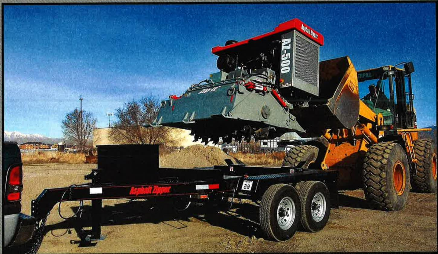
Asphalt Zipper's patented Versa-Mount™ universal bucket mounting system allows the Zipper to fit the widest possible range of loaders, backhoes, and skid steers. The Asphalt Zipper® mounts securely in just minutes. Optional quick-connect system also available.
