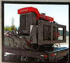
Asphalt Zipper's optional quick-connect system secures into the Versa-Mount™ bucket slot. Its side shift and tilt capability provides an impressive 36 inches of reach and 9 degrees of tilt, making profiling and grinding next to curbs a snap. Also, the quick-connect system can be removed when you want to use the Zipper on other loader buckets.
