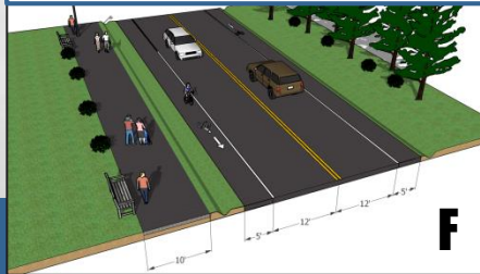
2 Lane Section With Bike Lanes, Pedestrian Pathway & No Curbs
