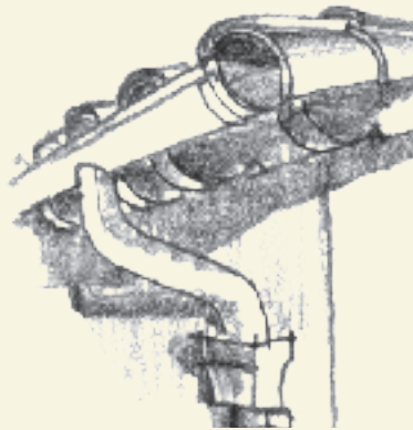
Rafter Tail and Downspout
