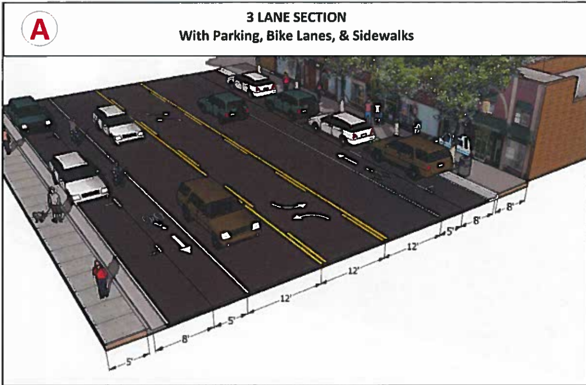
Figure 8B – Roadway Cross-Sections
