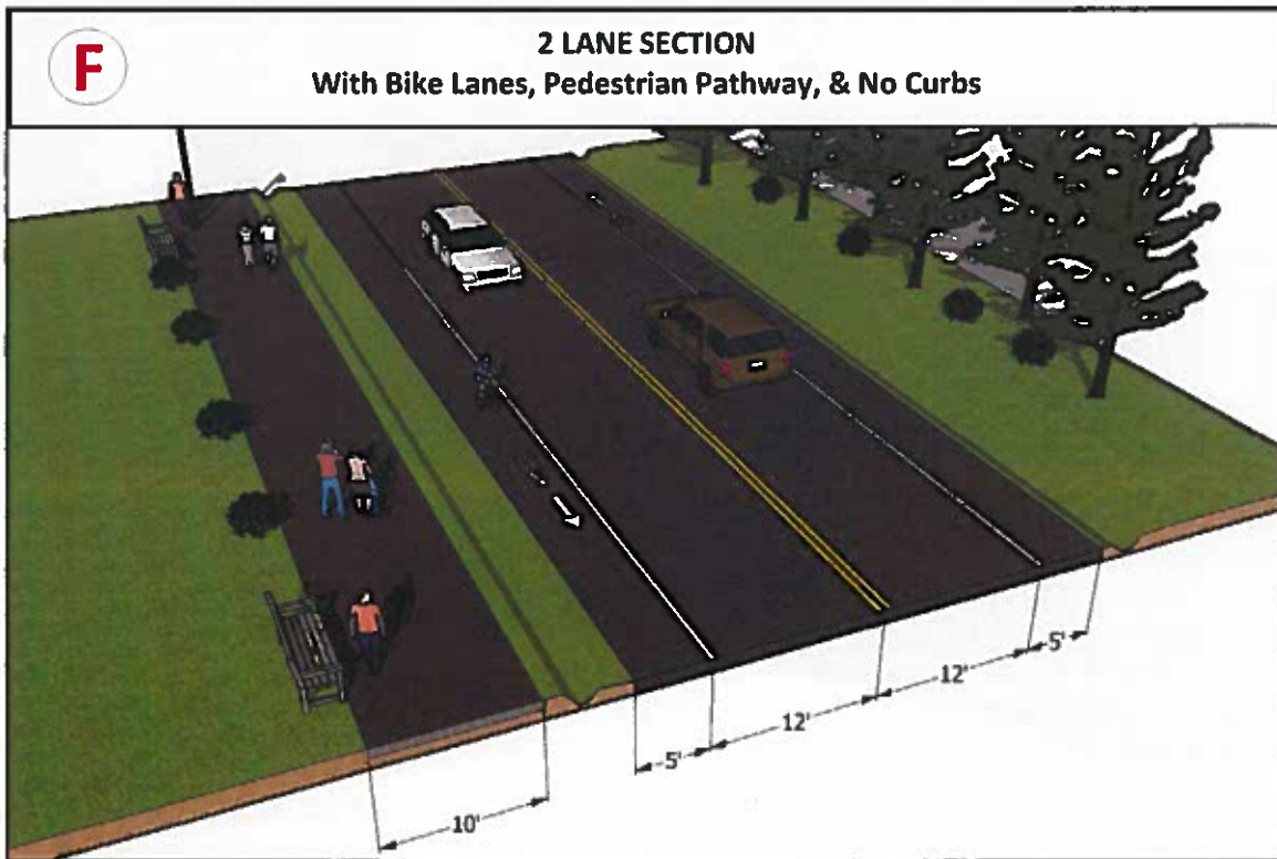
Figure 8F – Roadway Cross-Sections
