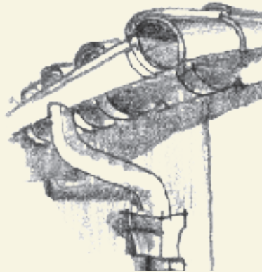
Rafter Tail and Downspout
