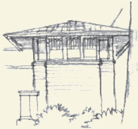
Massing with Hip Roof Form
