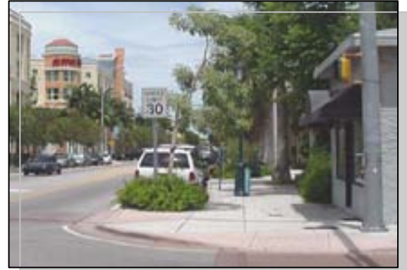
Example: Neckdown at intersection.
