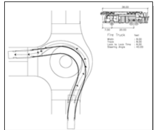
Example: Truck turning radius using mountable apron.
