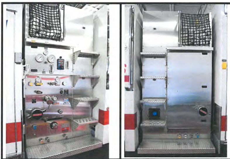
Figure 12: Fire Suppression Component of Combination Fire/EMS Transport Vehicle
