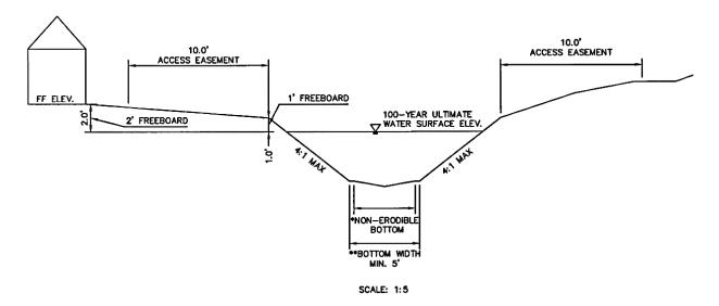
\*NON-ERODIBLE BOTTOM SHALL BE DESIGNED BY THE ENGINEER AND DOCUMENTATION AND CALCULATIONS SHALL BE PROVIDED TO CITY STAFF FOR REVIEW. GRADES SHALL ENSURE POSITIVE DRAINAGE THROUGHOUT THE CHANNEL.
