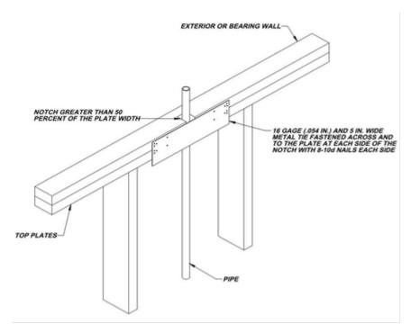
(Amendment to 2012 IRC carried forward to 2015 IRC also provides additional assurance of maintaining the integrity of the framing by spreading the nailing pattern.)
