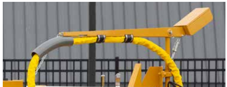
Ergonomic counter balanced hose boom
