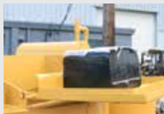
Anti-Splash Material Loading Hatch
