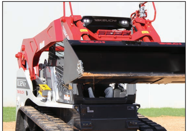
Vertical Lift Path for Balance and Stability
