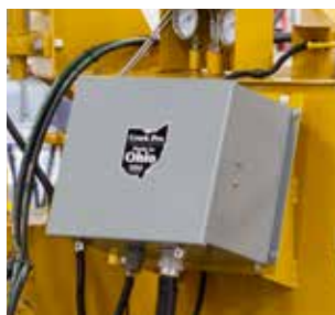
Steel enclosure for the control box
