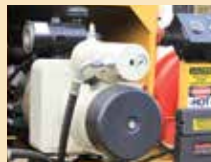
Direct Drive Air Compressor
