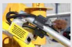
Horn button on wand
