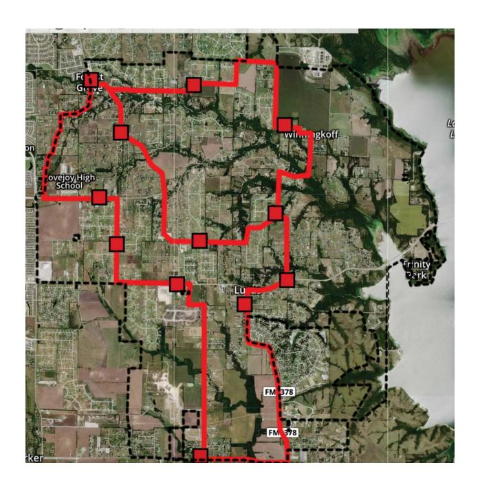
Figure 2: Lucas TX FTTP Distribution Network – 462,800 feet (87.7 Miles) UG Construction
