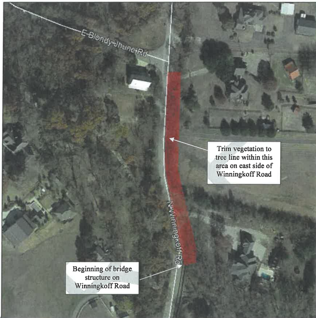
Figure 10: Additional Vegetation to Trim and Maintain on East Side of Winningkoff Road
