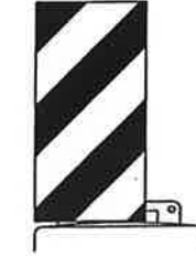
12" x 24" Vertical Panel mount with diagonals sloping down towards travel way
