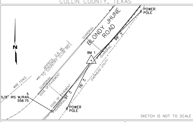
GENERAL DESCRIPTION: 3" BRASS CAP SET IN CONCRETE. BM1 IS LOCATED ON BLONDY JHUNE ROAD APPROXIMATELY 0.6 MILES EAST OF THE INTERSECTION OF BLONDY JHUNE ROAD AND COUNTRY CLUB ROAD. BM1 IS LOCATED 99 ± FEET SOUTHWEST OF A POWER POLE, 91 ± FEET NORTHEAST OF A 5/8" IRON ROD SET AND 76 ± FEET NORTHEAST OF A POWER POLE.
