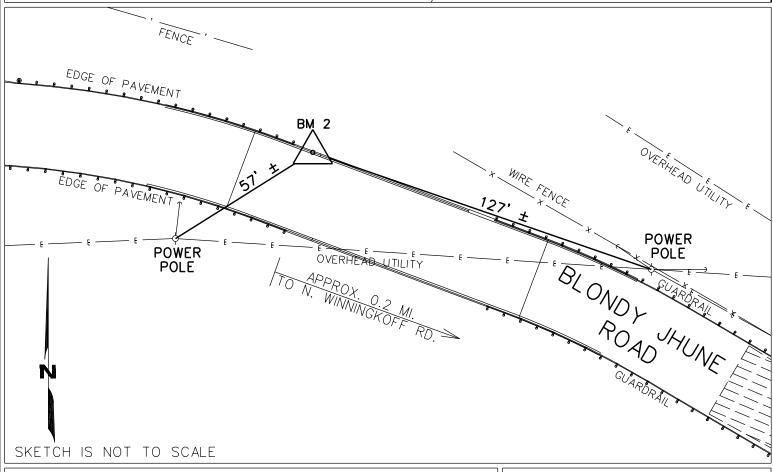
GENERAL DESCRIPTION: 3" BRASS CAP SET IN CONCRETE. BM2 IS LOCATED ON BLONDY JHUNE ROAD APPROXIMATELY 0.2 MILES WEST OF THE INTERSECTION OF BLONDY JHUNE ROAD AND NORTH WINNINGKOFF ROAD. BM2 IS LOCATED 127 ± FEET NORTHWEST OF A POWER POLE AND 57 ± FEET NORTHEAST OF A POWER POLE.
