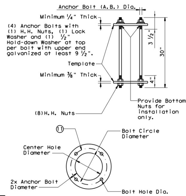
**TRANSFORMER BASE ANCHOR BOLT ASSEMBLY**
