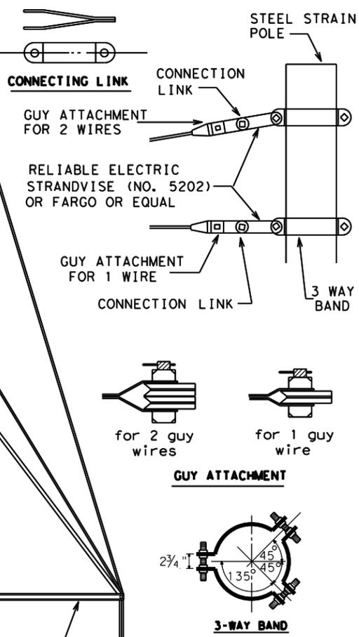
**SPAN CABLE ATTACHMENT
