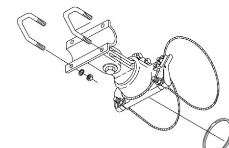
SHALL BE INSTALLED WHEN ROTATION ABOUT THE HORIZONTAL AND VERTICAL AXES ARE NEEDED.
