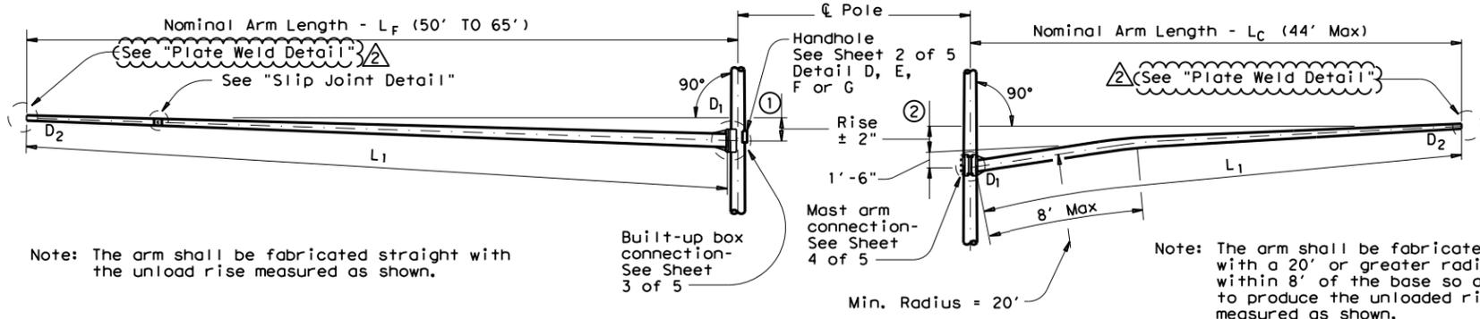
Note: The arm shall be fabricated straight with the unload rise measured as shown.
