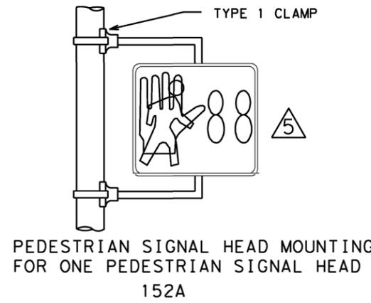
PEDESTRIAN SIGNAL HEAD MOUNTING FOR ONE PEDESTRIAN SIGNAL HEAD 152A
