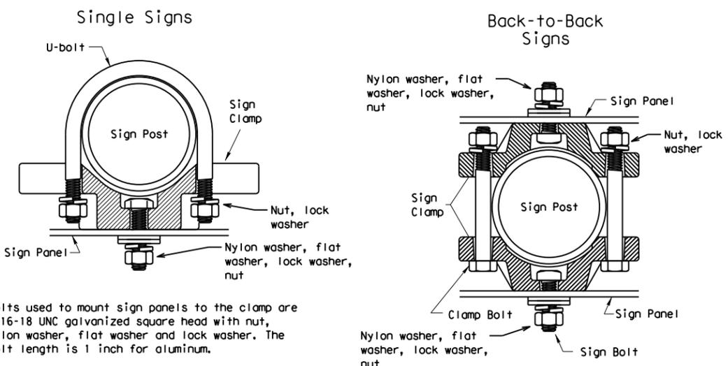
Bolts used to mount sign panels to the clamp are 5/16-18 UNC galvanized square head with nut, nylon washer, flat washer and lock washer. The bolt length is 1 inch for aluminum.
