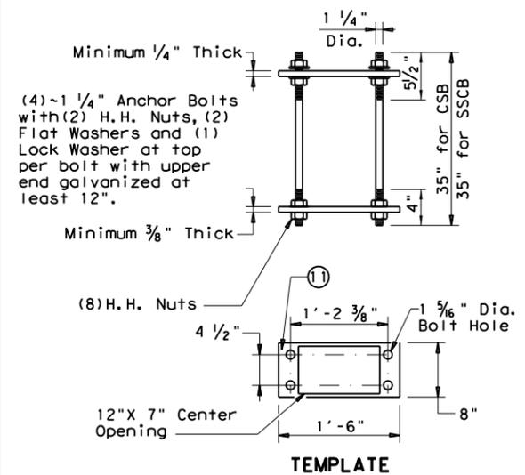
**CONCRETE TRAFFIC BARRIER BASE ANCHOR BOLT ASSEMBLY**
