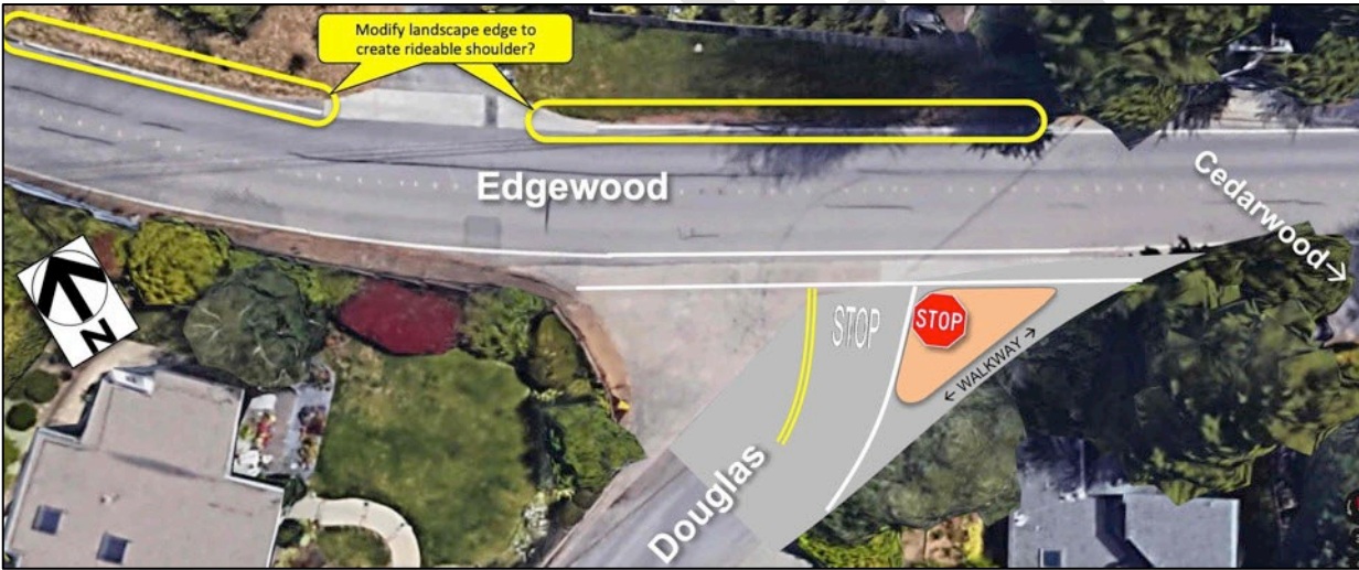
Figure 4-21: Edgewood Avenue / Douglas Drive Intersection – Concept
