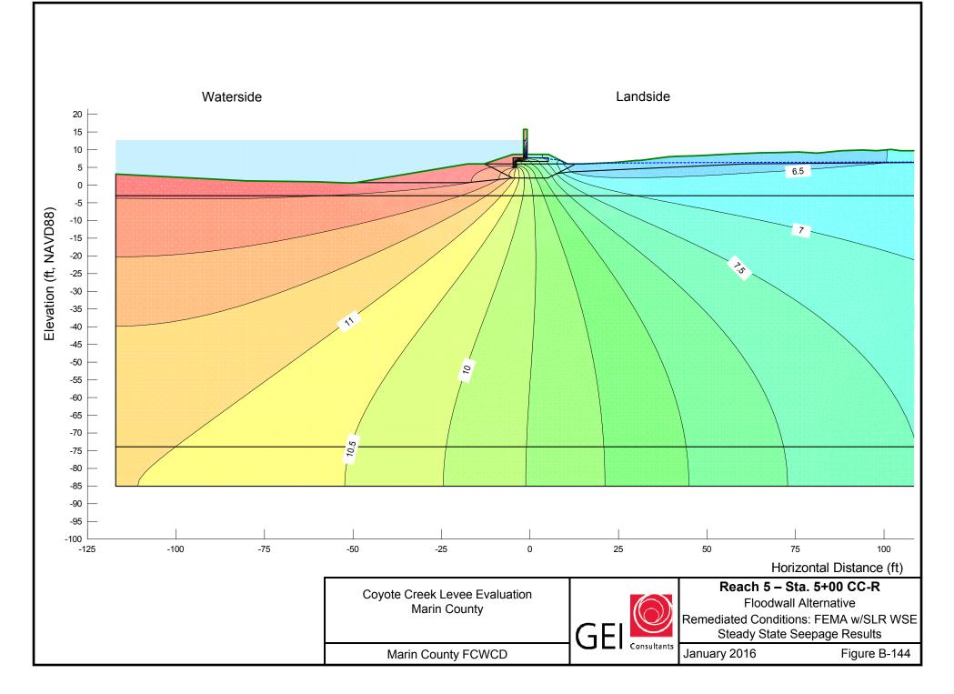
5+00 CC-R\_Reach 5 – Floodwall – All DWSEs\_2\_1\_0\_Stability\_Model
