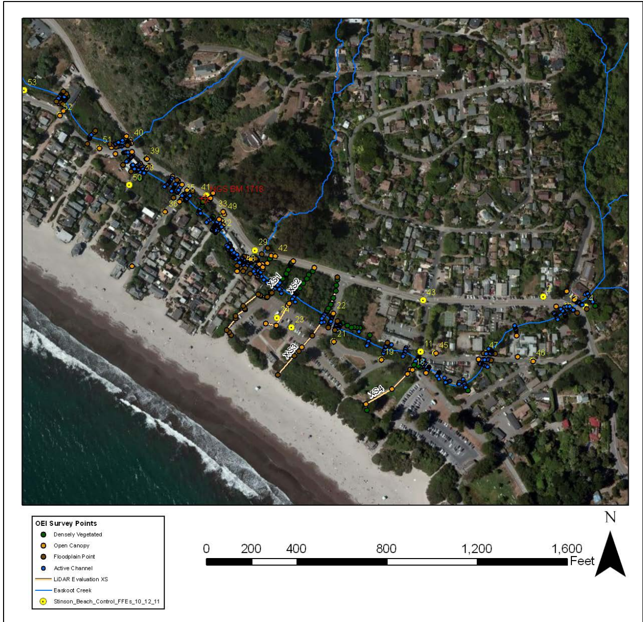
Figure B1 Overview map showing the locations of the OEI survey points, control points, and cross sections used in the LiDAR evaluation.
