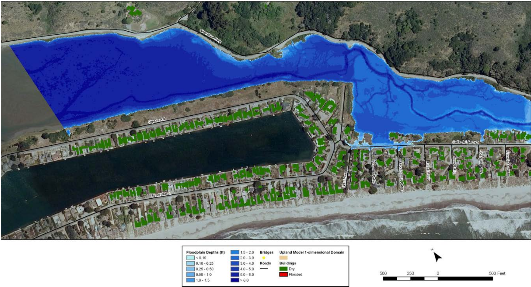
Figure D13B Maximum inundation depths during the January 2008 event (lower reach).
