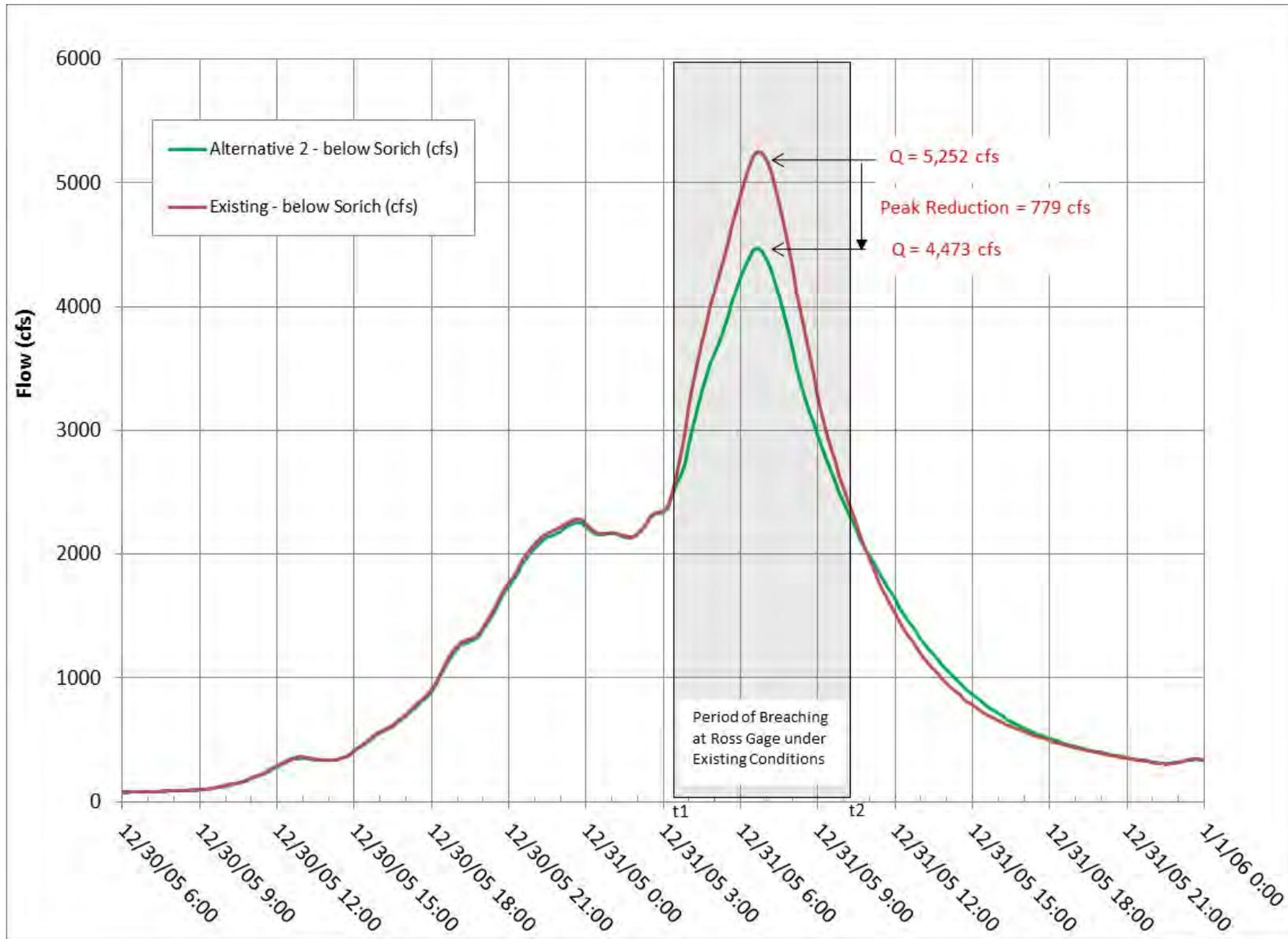
Figure 13 Peak Flow Reduction at Ross Gage - Alternative 2
