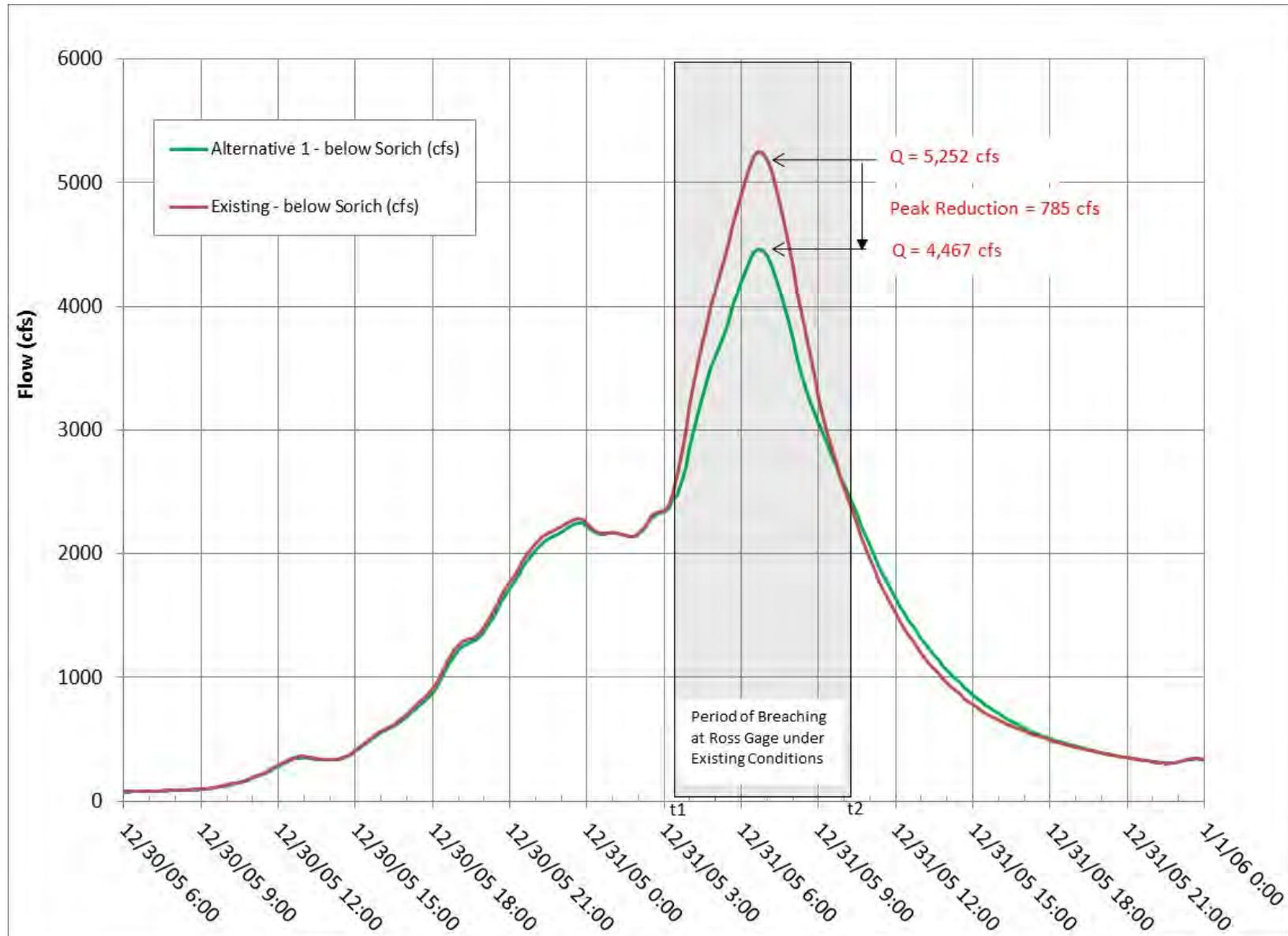
Figure 10 Peak Flow Reduction at Ross Gage - Alternative 1
