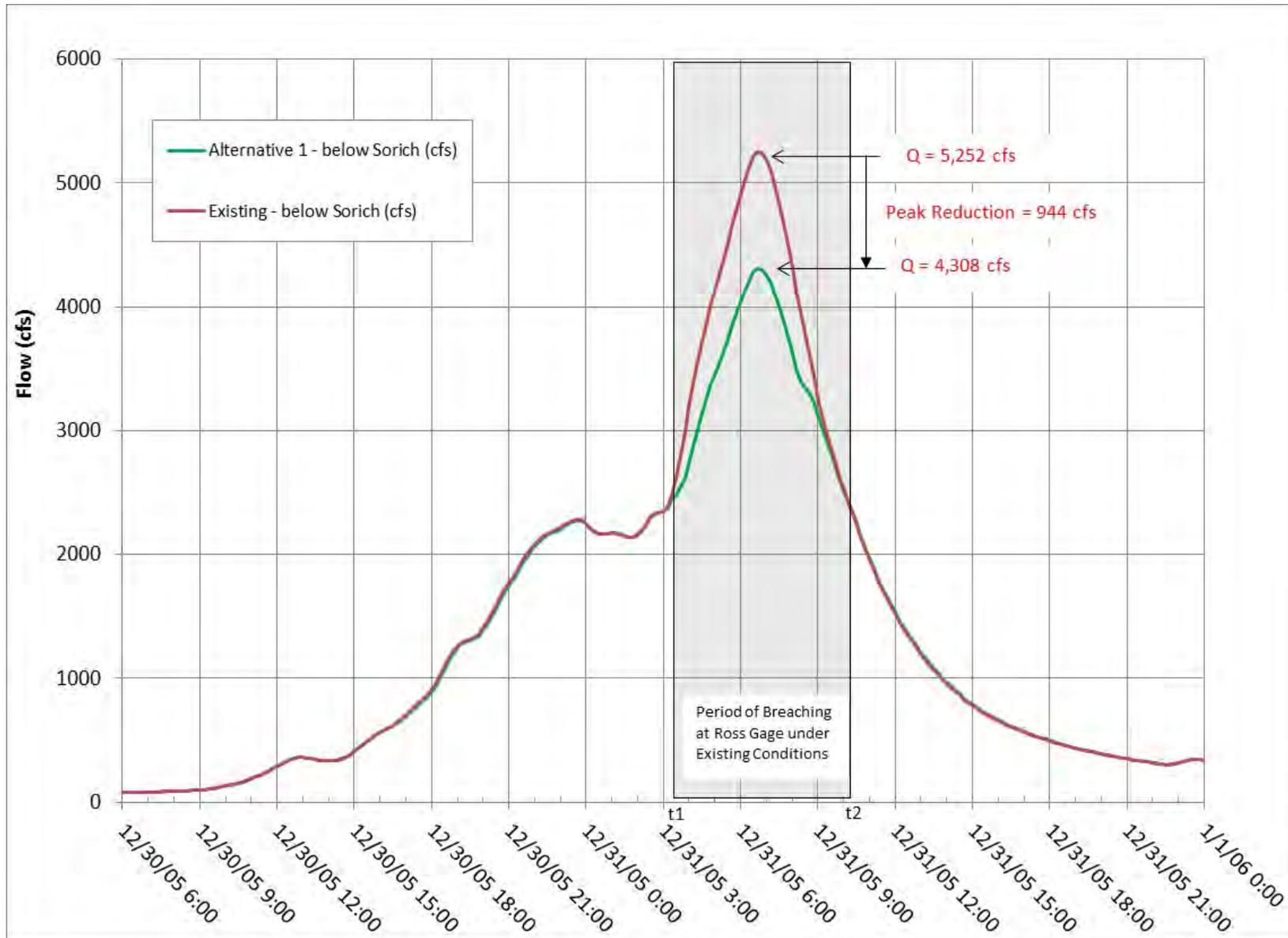
Figure 16 Peak Flow Reduction at Ross Gage - Alternative 3
