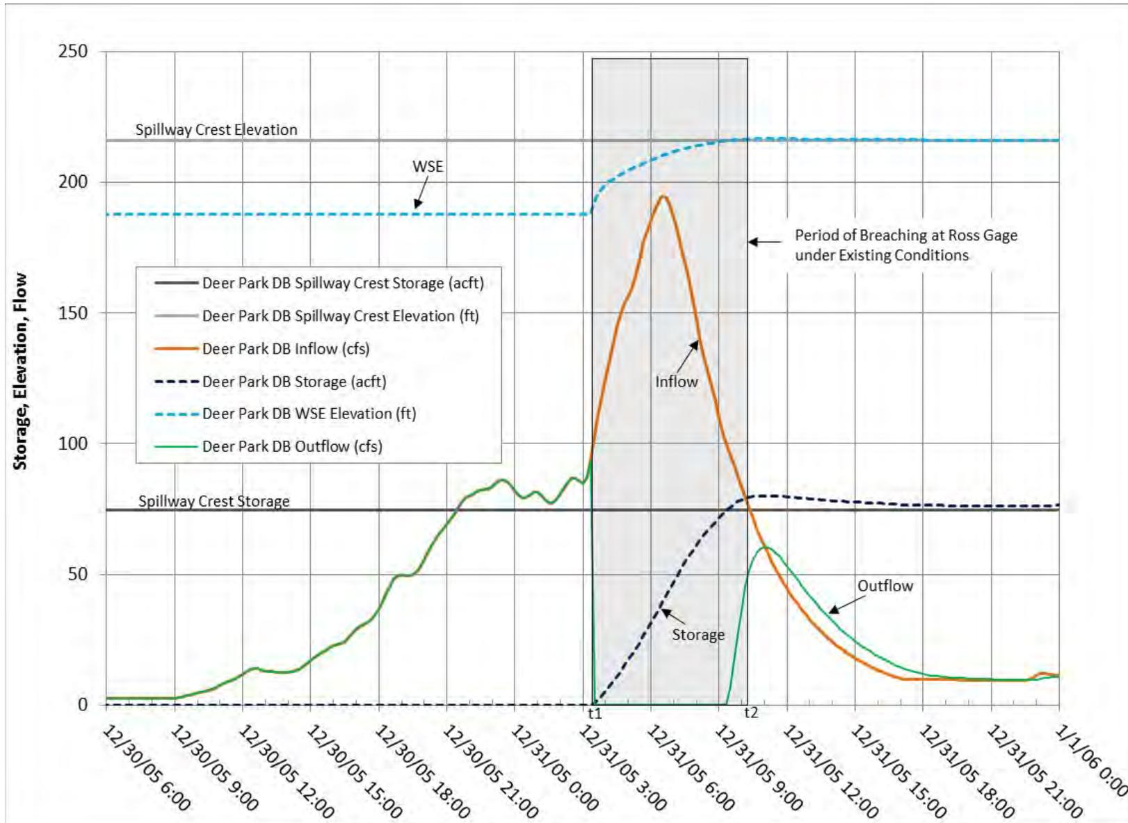
**Figure 4 Simulated Hydrographs of San Domenico Detention Basin During the Design Flood Event of 12/31/2005**
