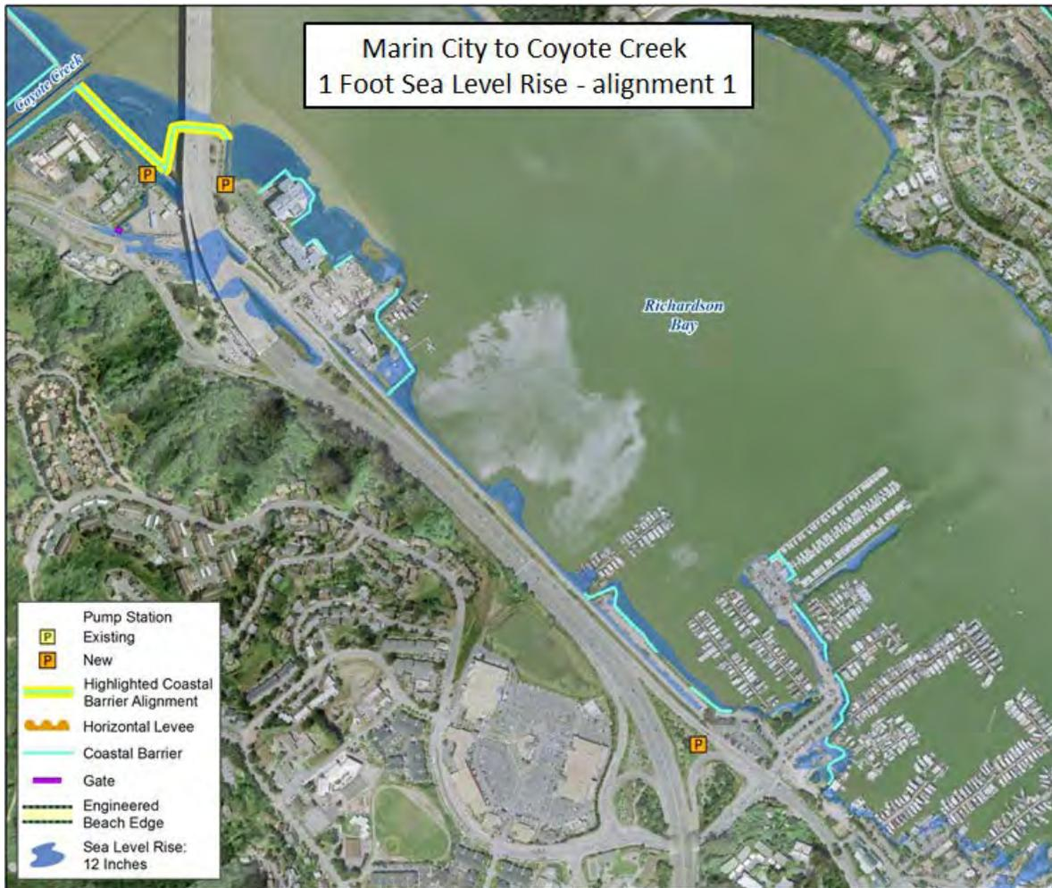
**Figure 30: Reach 1, Alignment 1. Extent of Direct Coastal Flooding Barrier 12 Inch Sea Level Rise Scenario.**
