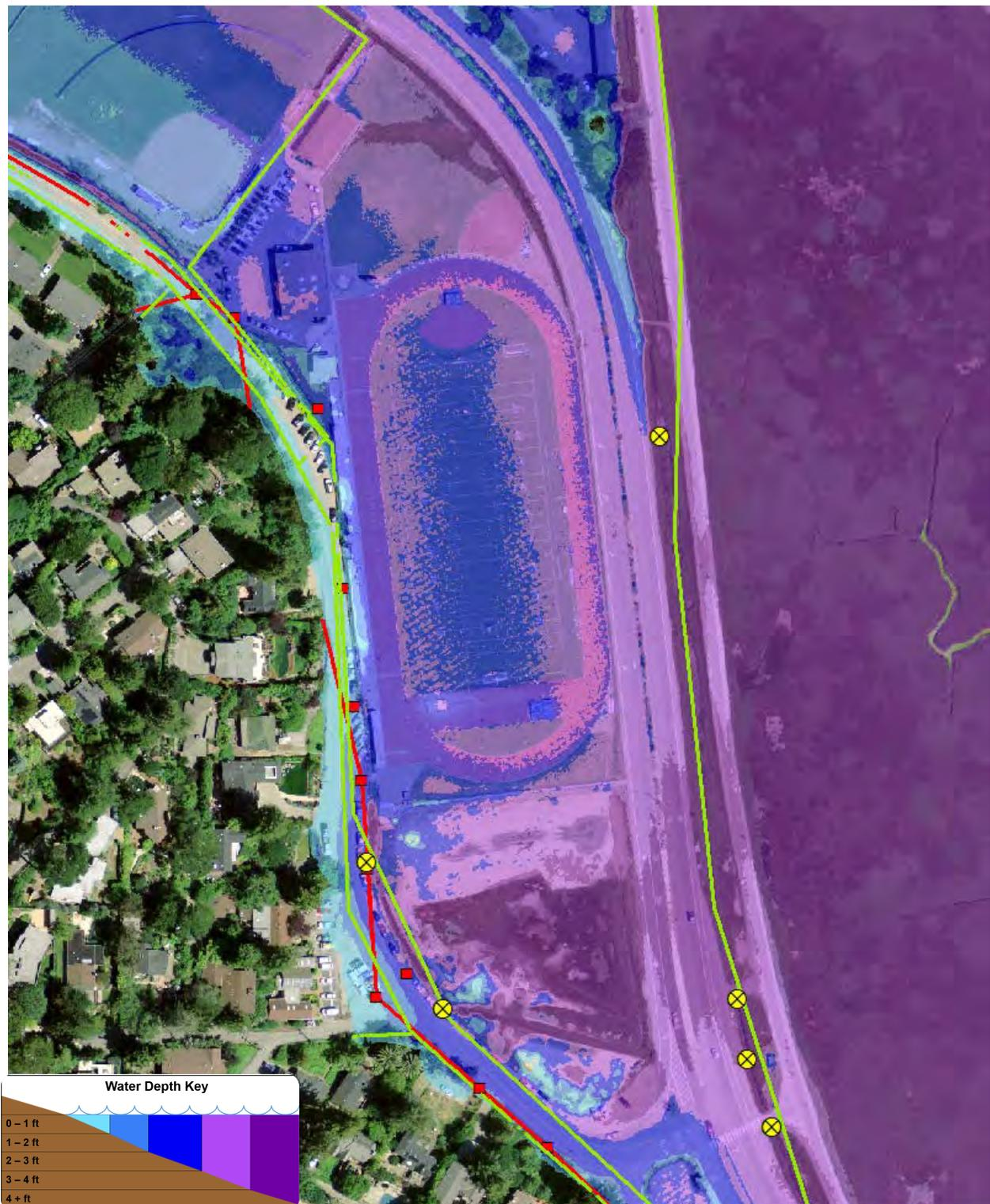
**Figure 29: Flooding Across Miller Avenue. 60 Inch Sea Level Rise Assuming No Mitigation Measures; Flooding Depths on the Order of 3 to 4 Feet Across Roadway.**
