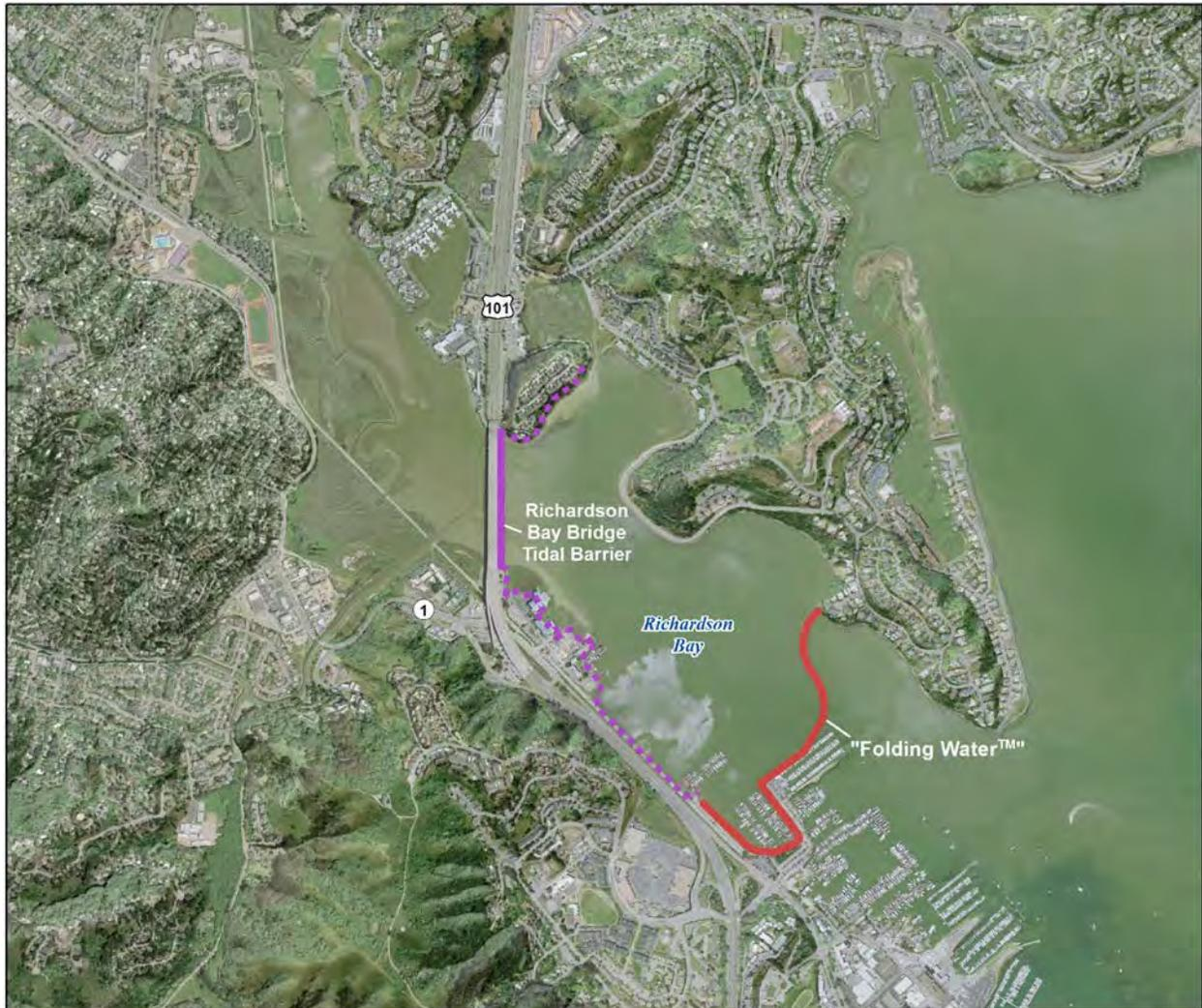
**Figure 39: Locations of Two Proposed High Tide Barriers at the Entrance to Richardson Bay.**
