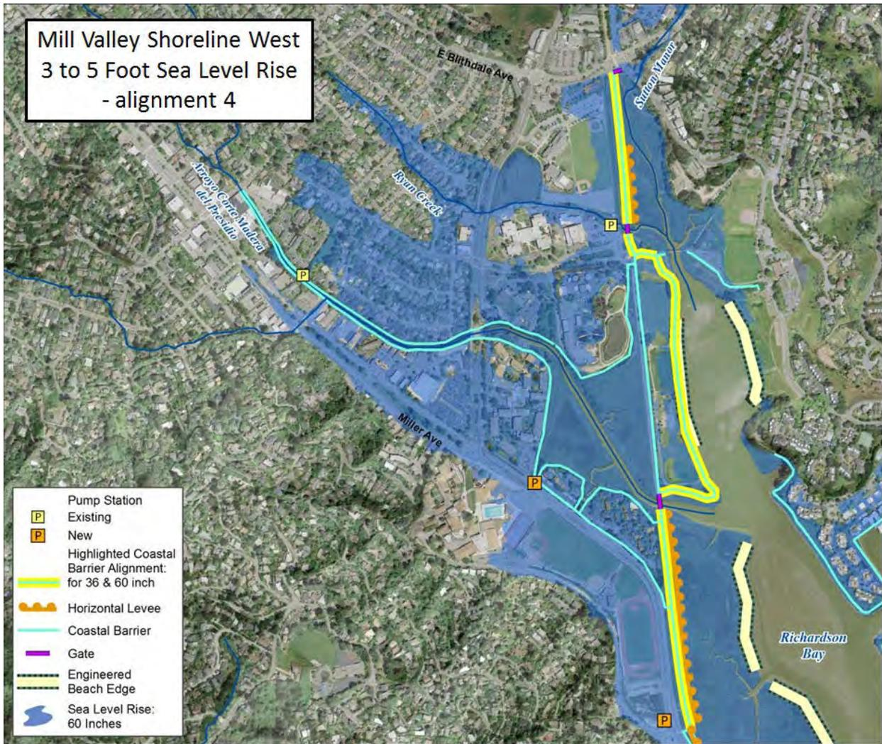
**Figure 49: Reach 3, Alignment 4. 36 and 60 Inch Sea Level Rise Alignment.**
