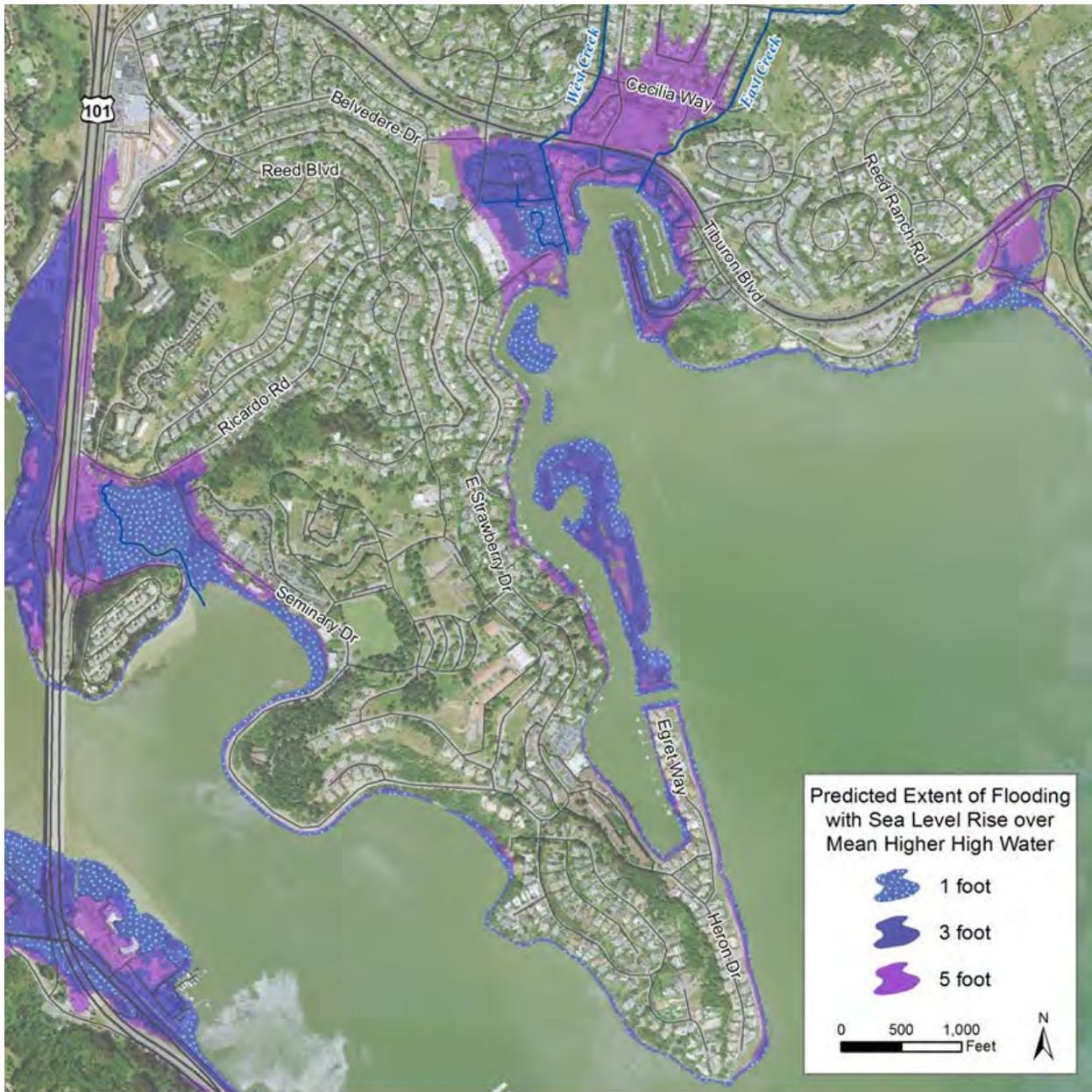
**Figure 15: Sea Level Rise Inundation Extents for Reaches 5 through 7.**
