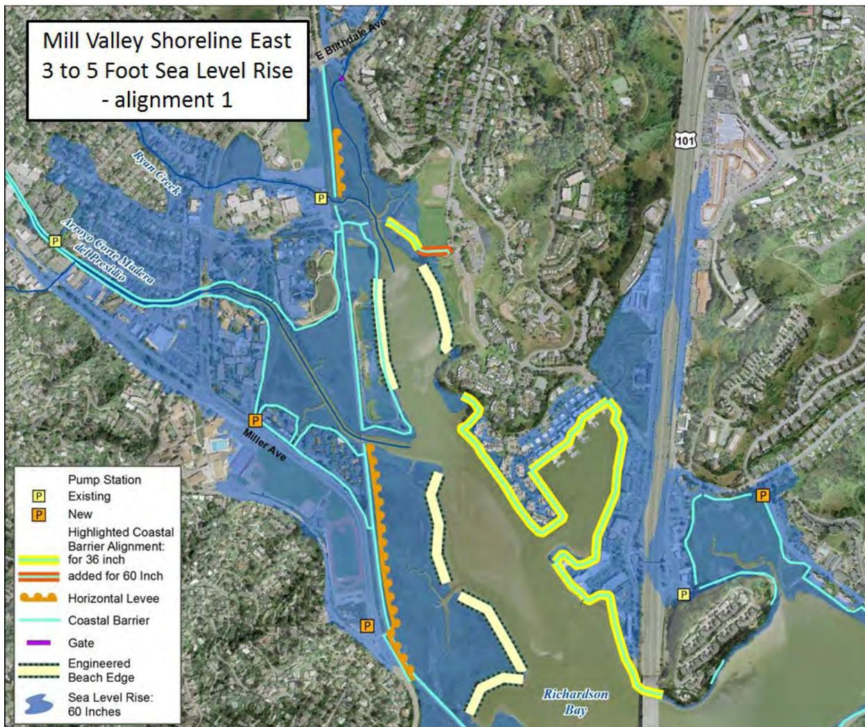
Figure 52: Reach 4, Alignment 1. 36 and 60 Inch LDCF Alignment.
