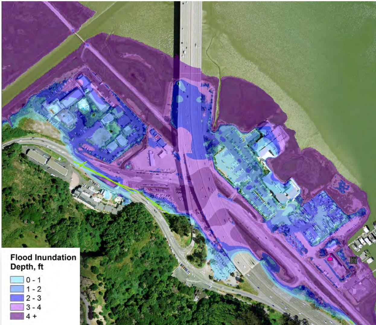
**Figure 22: Flood Focus, Manzanita Parking Area. 60 Inch Sea Level Rise.**
