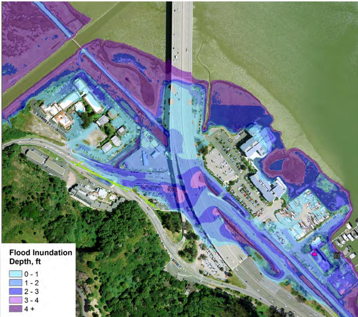
**Figure 21: Flood Focus, Manzanita Parking Area. 36 Inch Sea Level Rise.**
