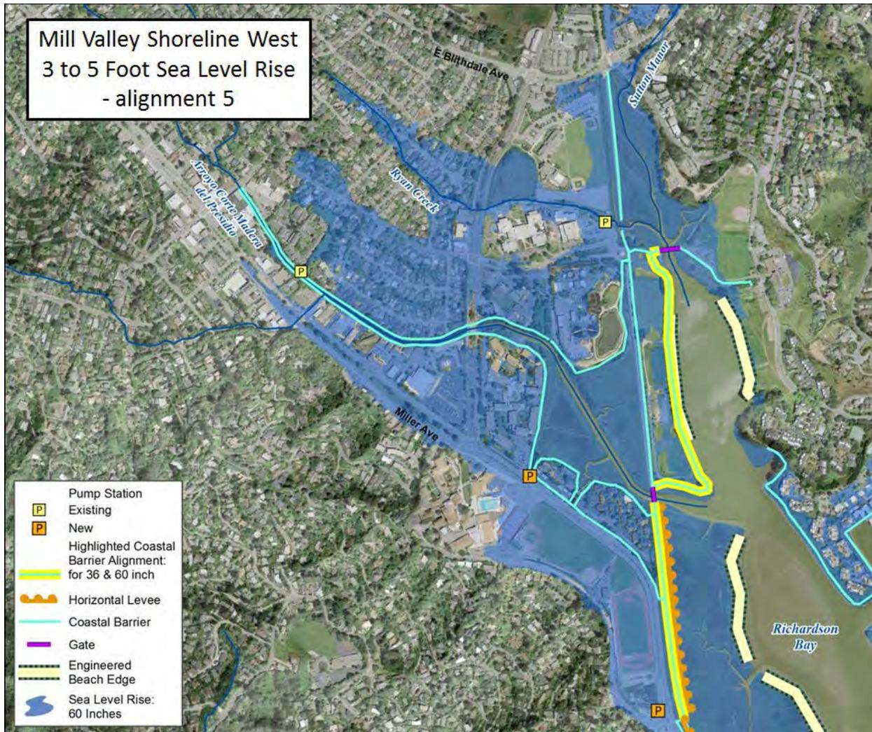
**Figure 50: Reach 3, Alignment 5. 36 and 60 Inch Sea Level Rise Alignments.**
