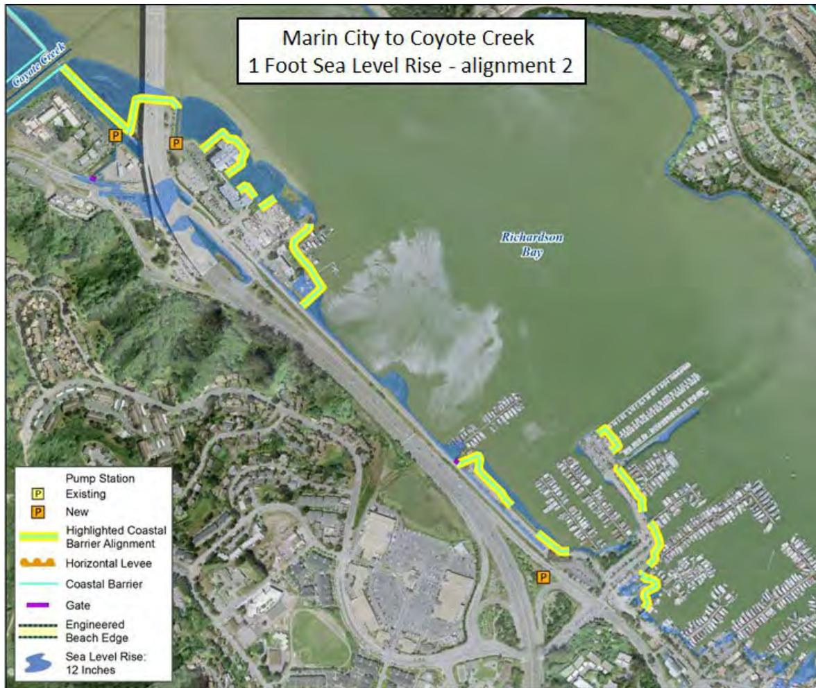
**Figure 31: Reach 1, Alignment 2. Potential Limit of Direct Coastal Flooding Barrier Alignment.**
