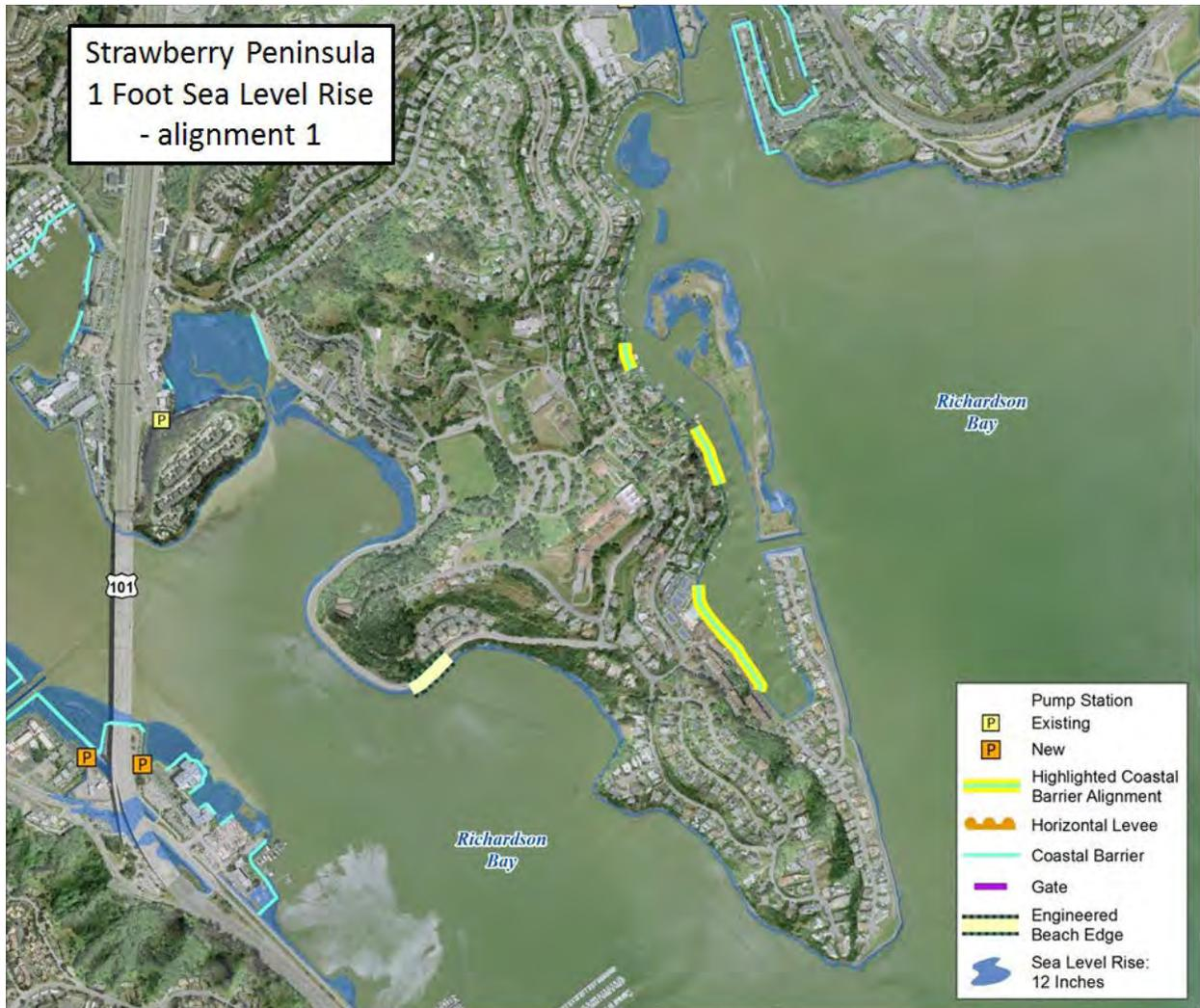
**Figure 37: Reach 6. Possible LDCF Barrier Alignment.**
