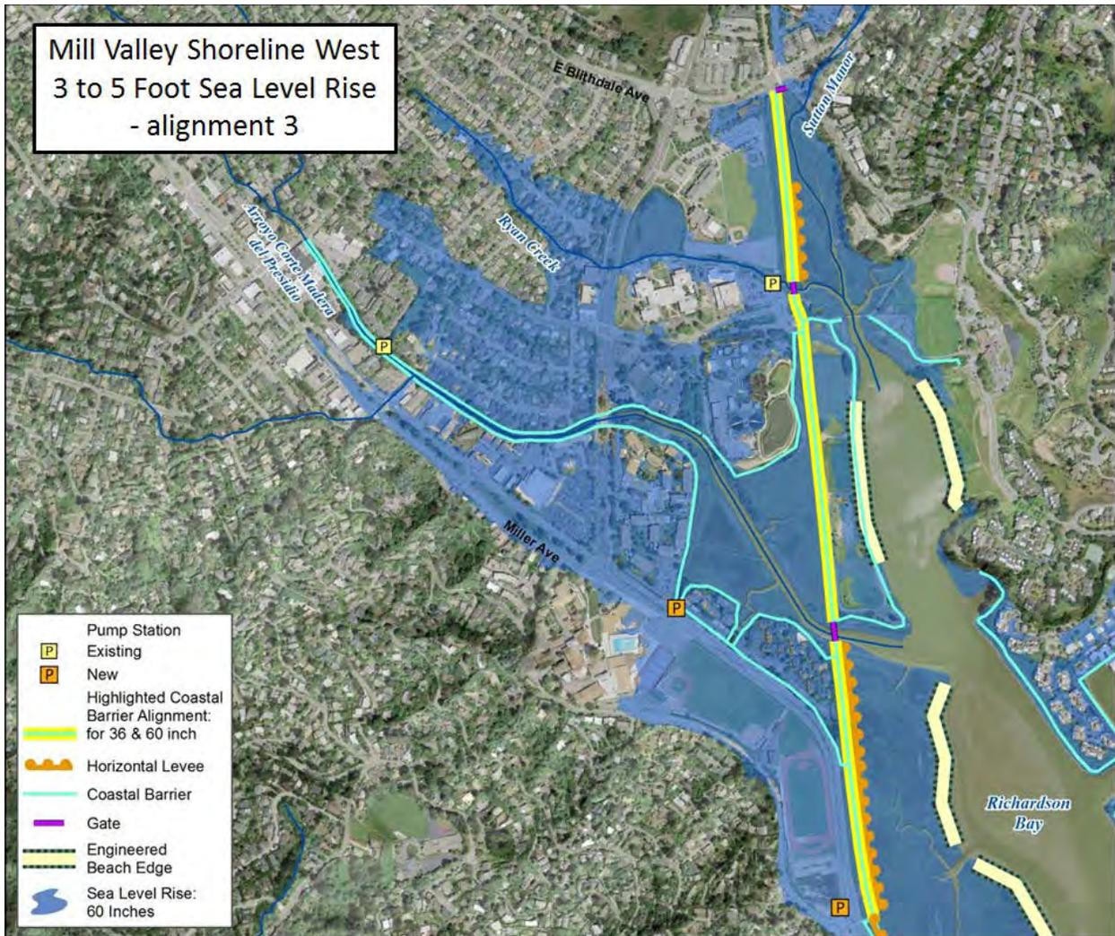
**Figure 48: Reach 3, Alignment 3. 36 and 60 Inch LDCF Alignment.**
