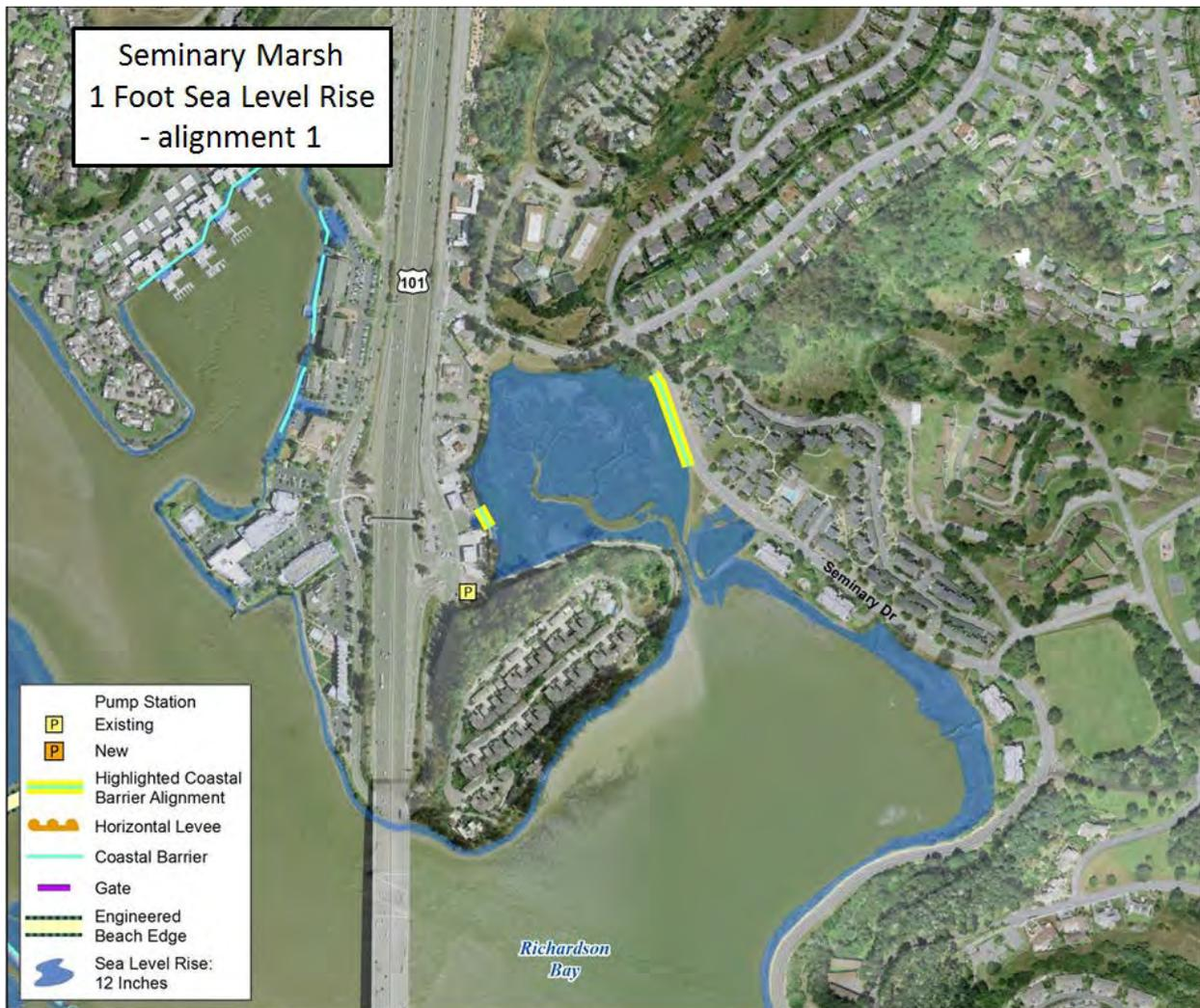
**Figure 36: Reach 5, Alignment 1. Possible LDCF Barrier Alignment.**
