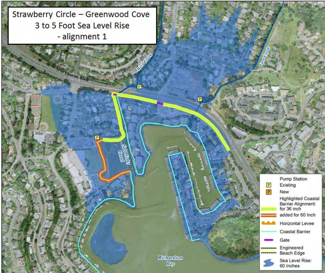
**Figure 55: Reach 7, Alignment 1. 36 and 60 Inch LDCF Alignment.**
