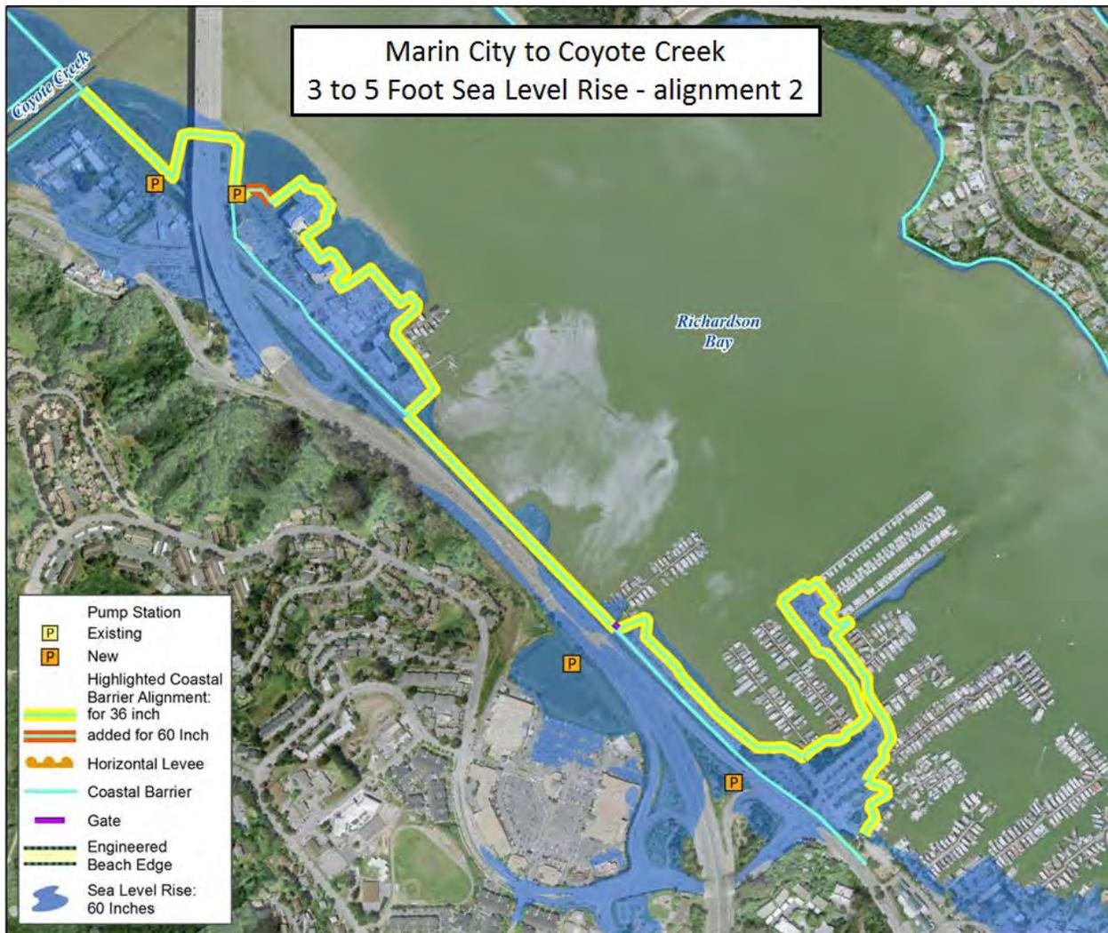
**Figure 41: Reach 1, Alignment 2. 36 and 60 Inch Sea Level Rise LDCF Alignments.**
