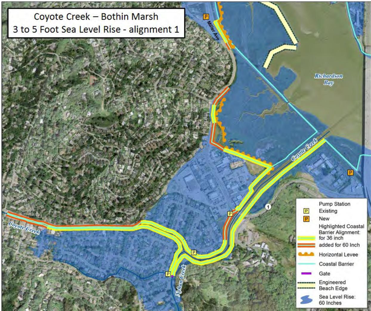
**Figure 42: Reach 2, Alignment 1. 36 and 60 Inch Sea Level Rise.**
