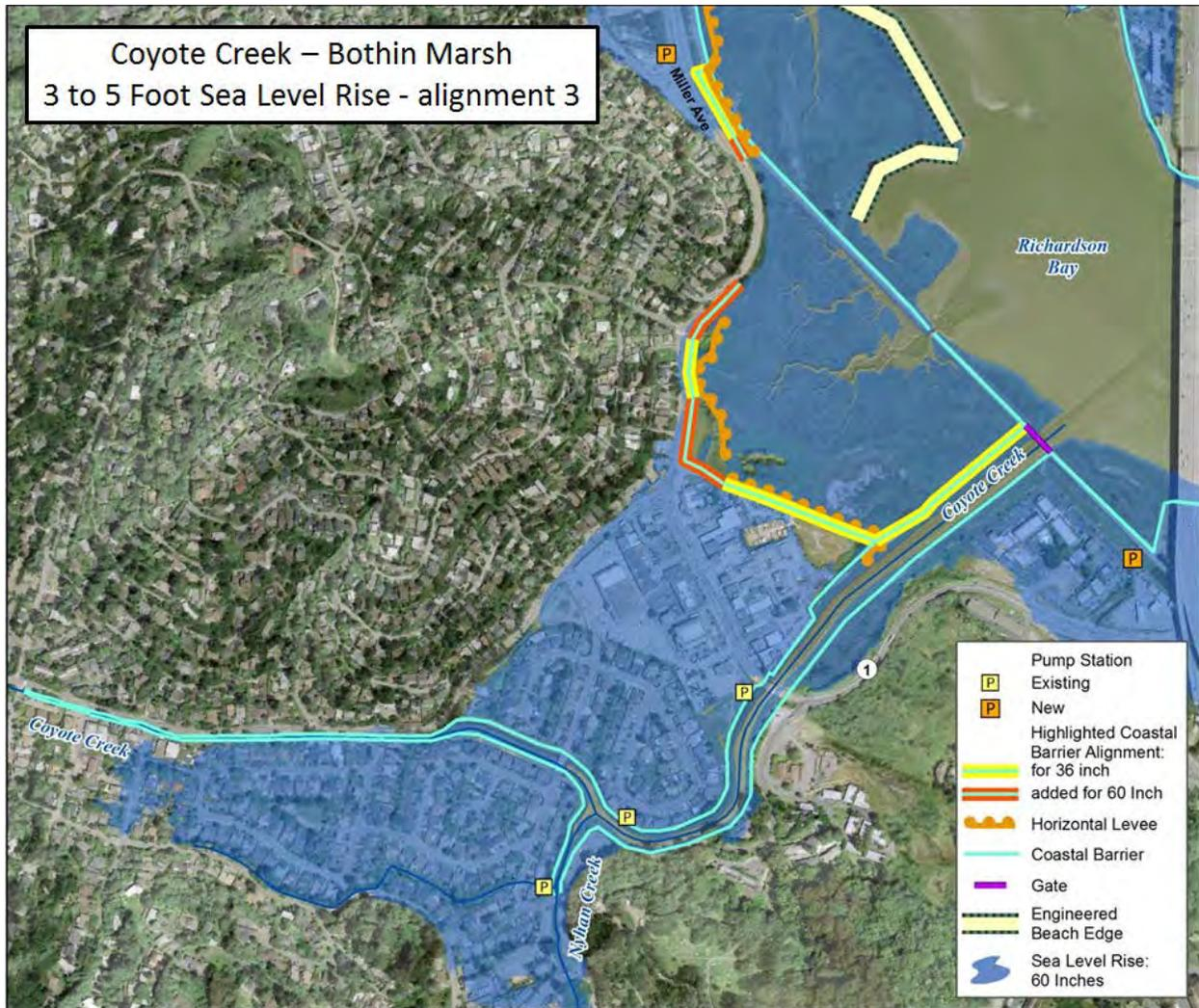
**Figure 44: Reach 2, Alignment 3. 36- and 60- Inch LDCF Alignments.**
