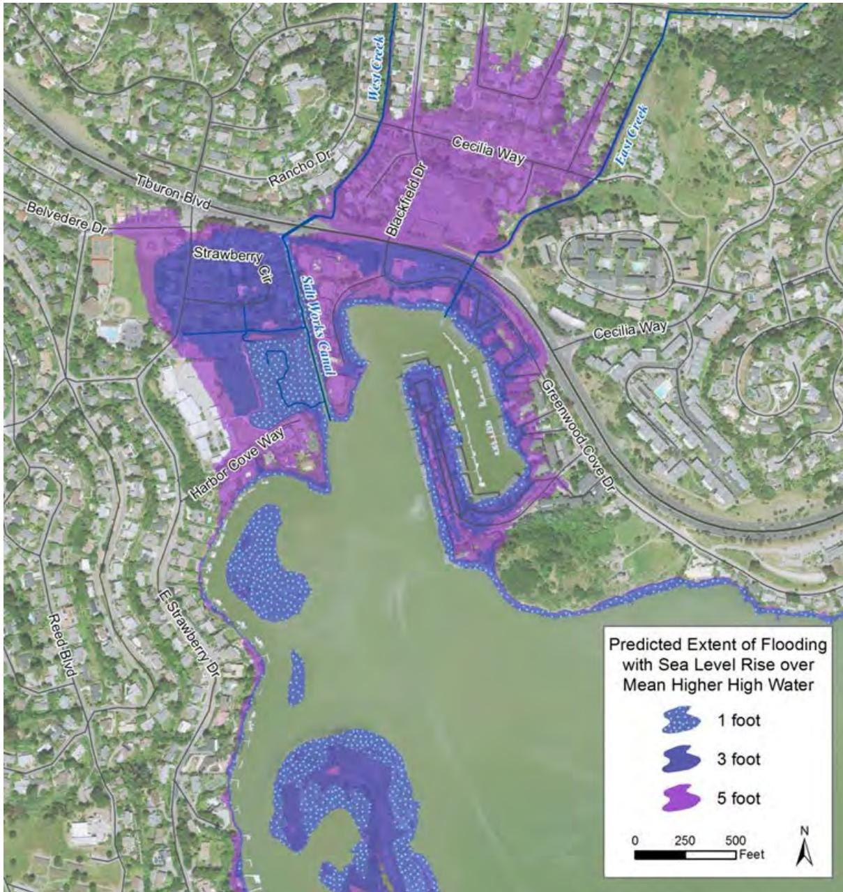
**Figure 16: Sea Level Rise Inundation Scenario Extents for Reaches 6 and 7.**
