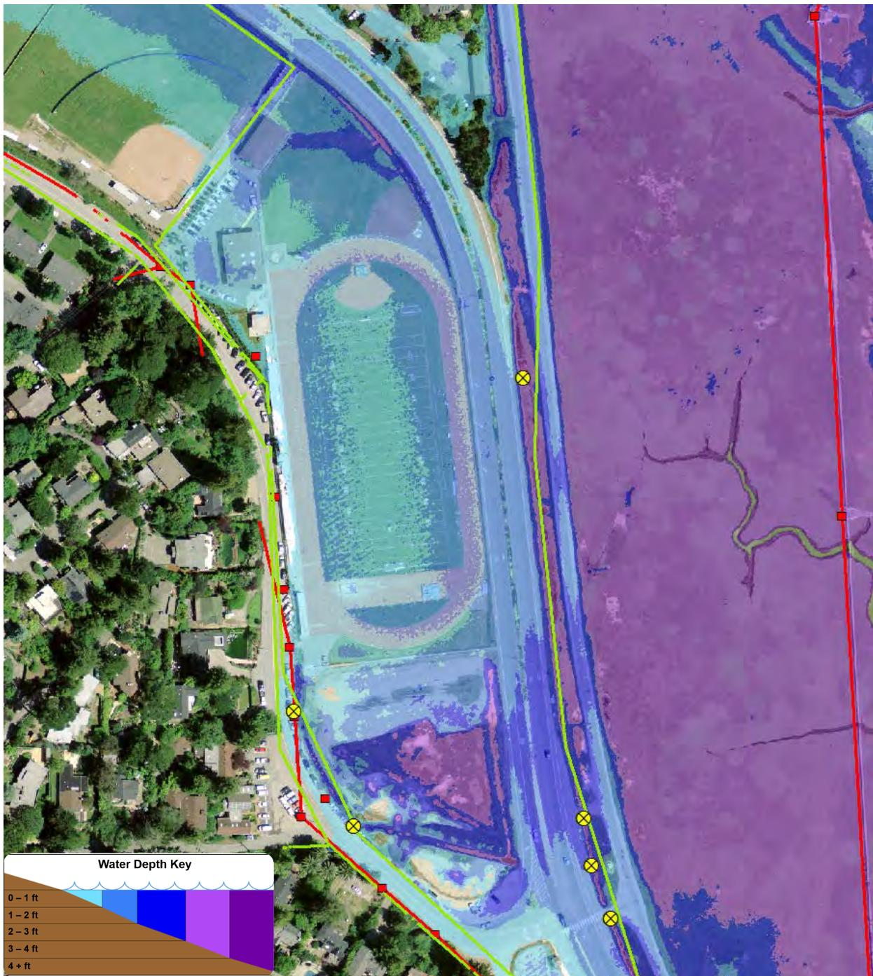
**Figure 28: Flooding Across Miller Avenue. 36 Inch Sea Level Rise Assuming No Mitigation Measures; Flooding Depths on the Order of 1 to 2 Feet Across Roadway.**
