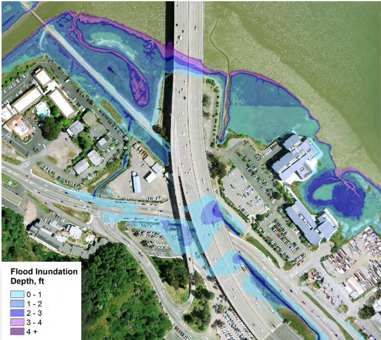
**Figure 17. Critical Area Inundation Focus Map Showing Flooding Depths with 12 Inches of Sea Level Rise at Shoreline Highway and Manzanita Parking Area South of Coyote Creek.**
