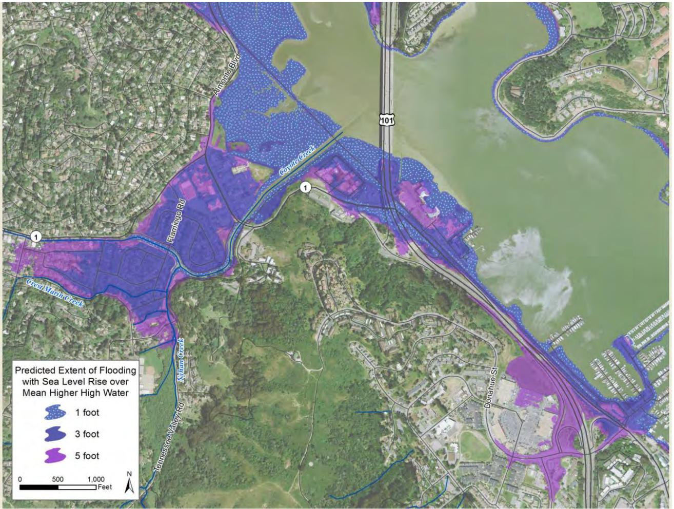
**Figure 13: Reach 1 and 2 Inundation Extents for Three Sea Level Rise Scenarios (12, 36, and 60 Inches).**
