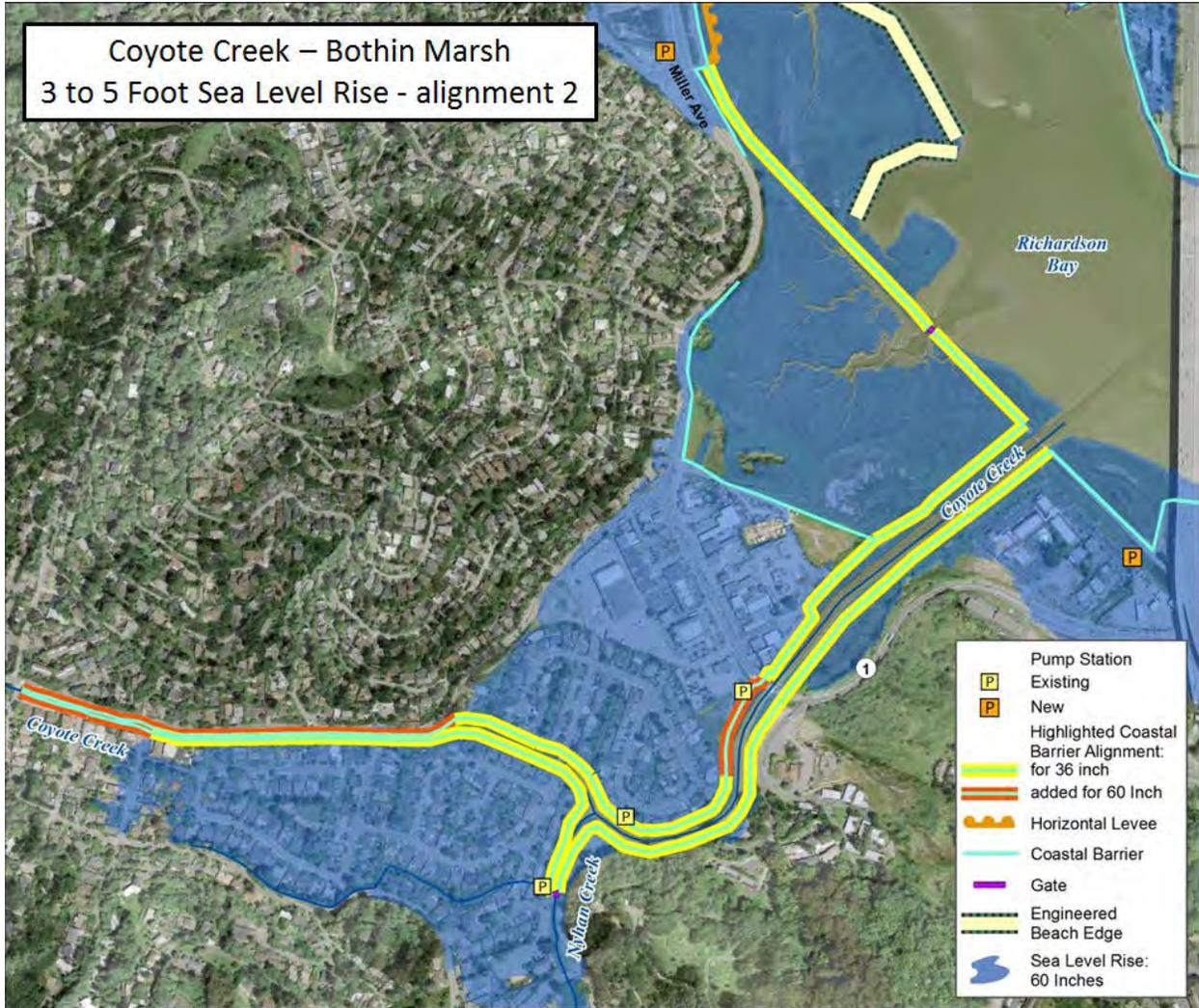
**Figure 43: Reach 2, Alignment 2. 36 and 60 Inch LDCF Alignments.**
