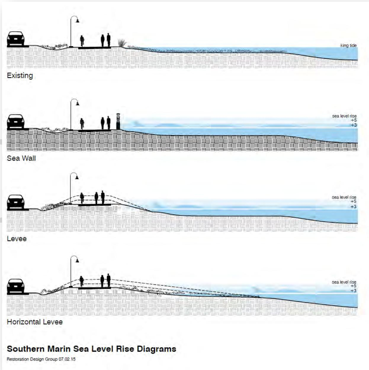
**Figure 51: Example Concept Cross-Sections of Miller Avenue with Different Adaptation Options under Varying Levels of Sea Level Rise.**
