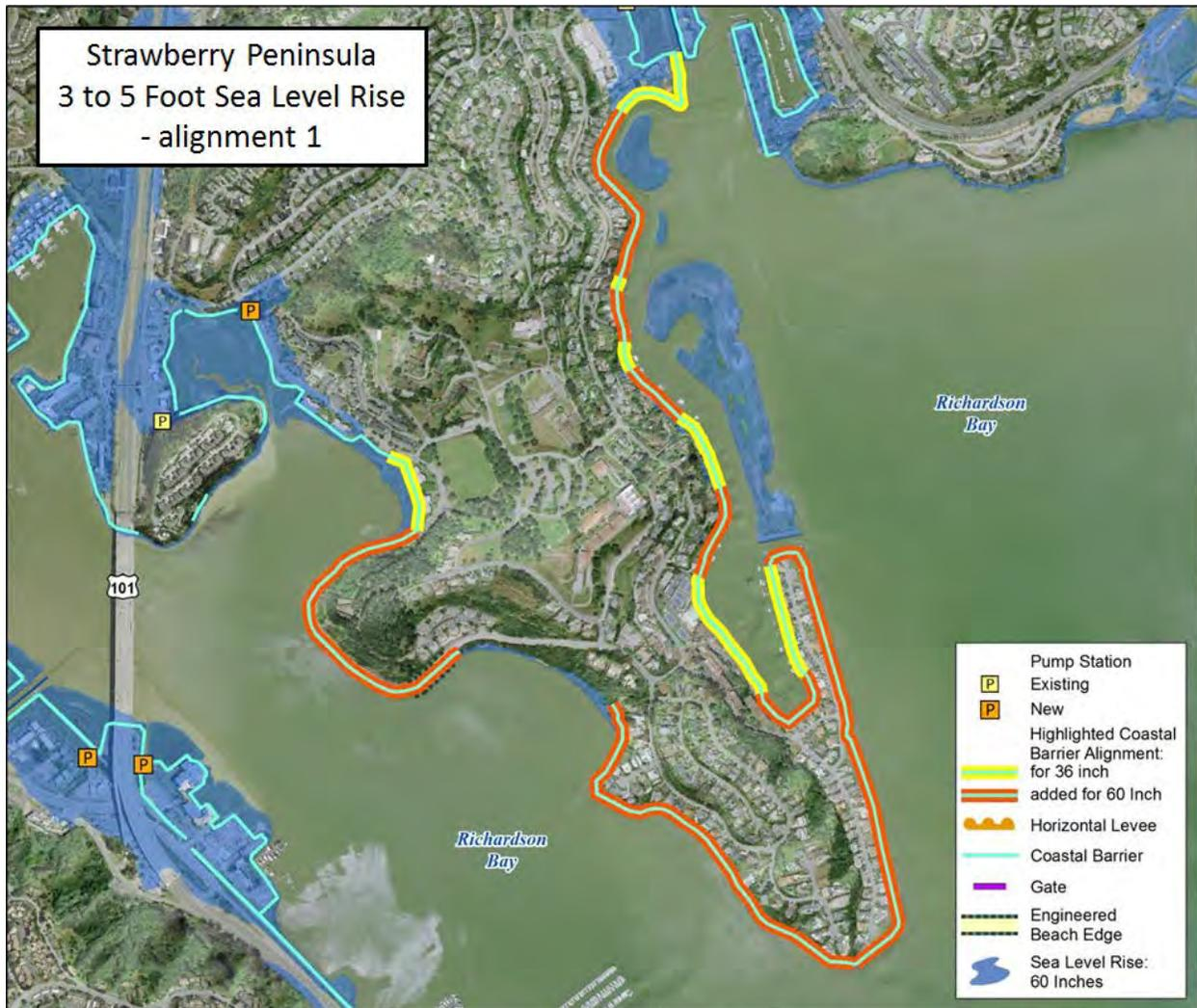
**Figure 54: Reach 6, Alignment 1. 36 and 60 Inch LDCF Alignment.**
