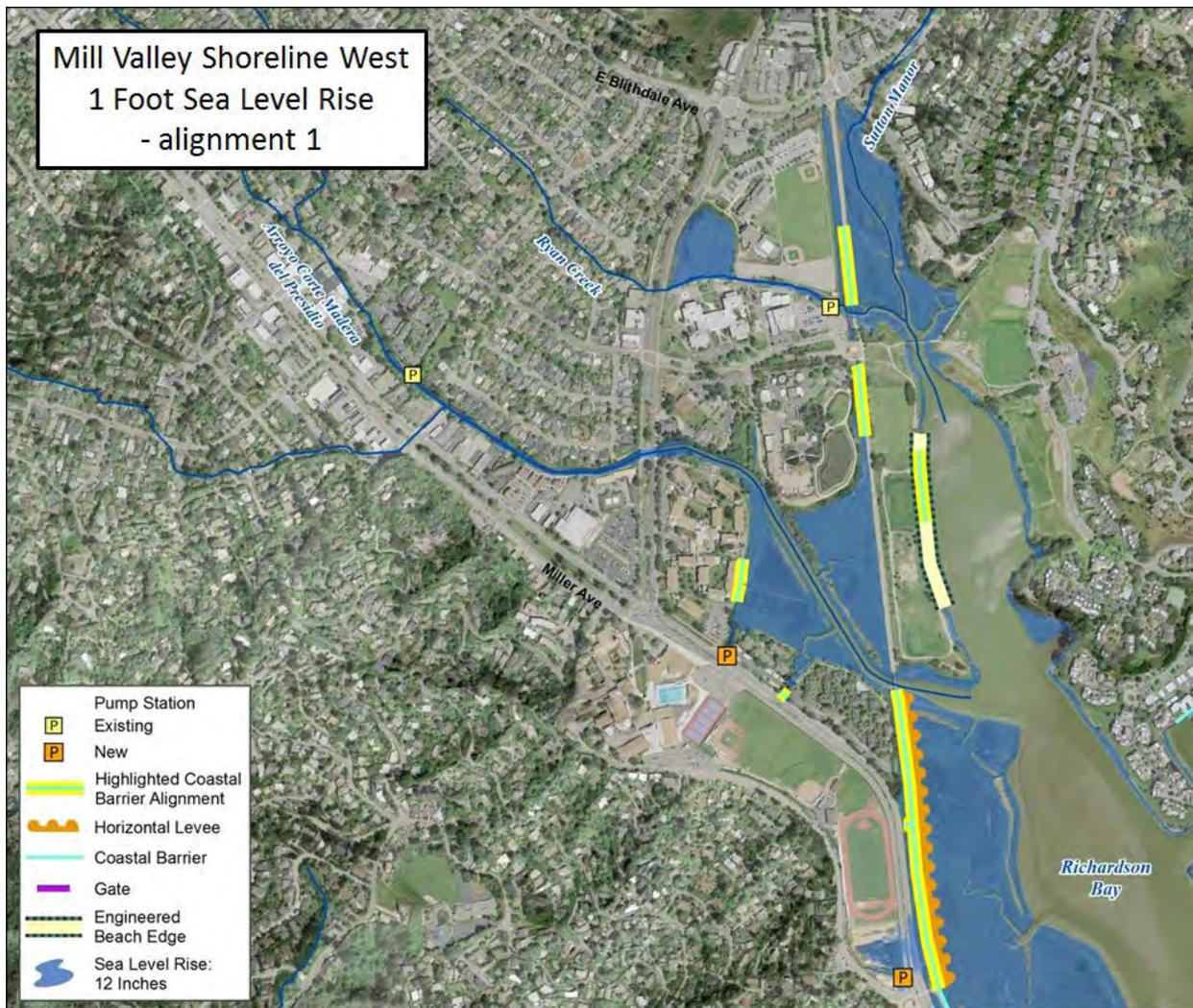
**Figure 34: Reach 3, Alignment 1. Possible LDCF Barrier Alignment.**
