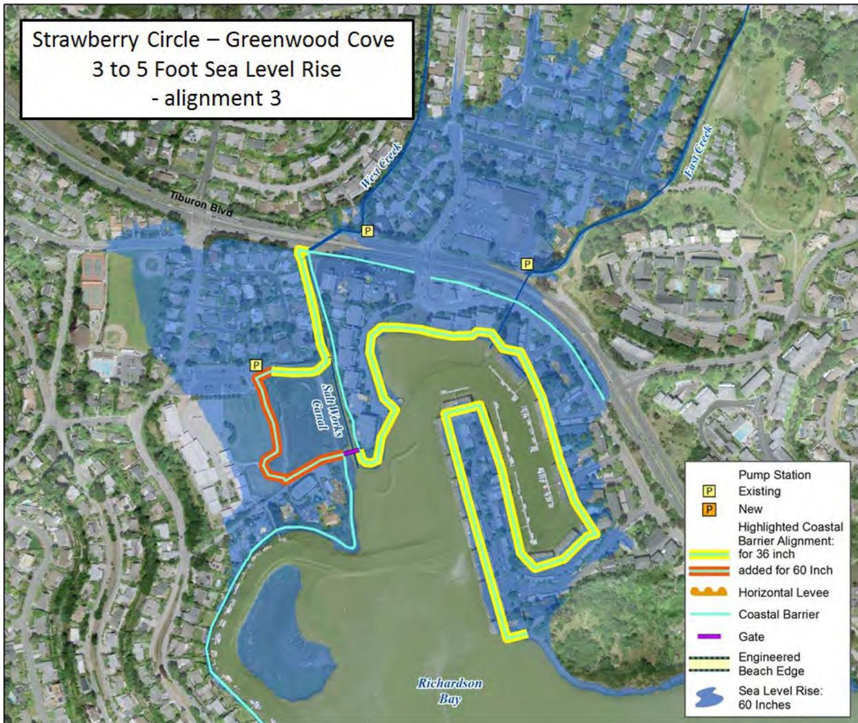
Figure 57: Reach 7, Alignment 3. 36 and 60 Inch LDCF Alignment.
