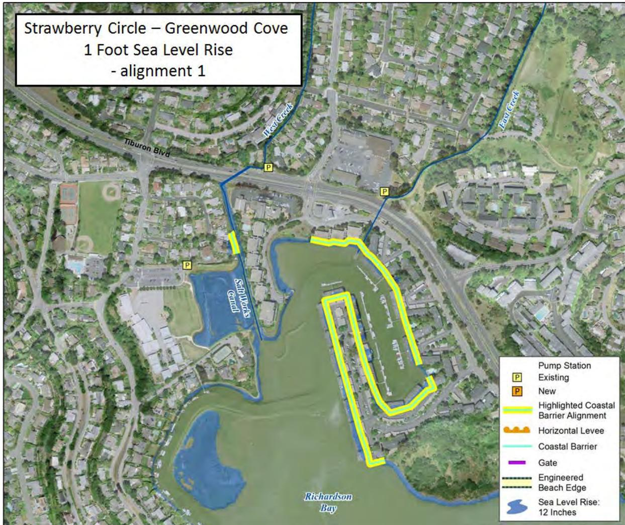
**Figure 38: Reach 7. Possible LDCF Barrier Alignment.**
