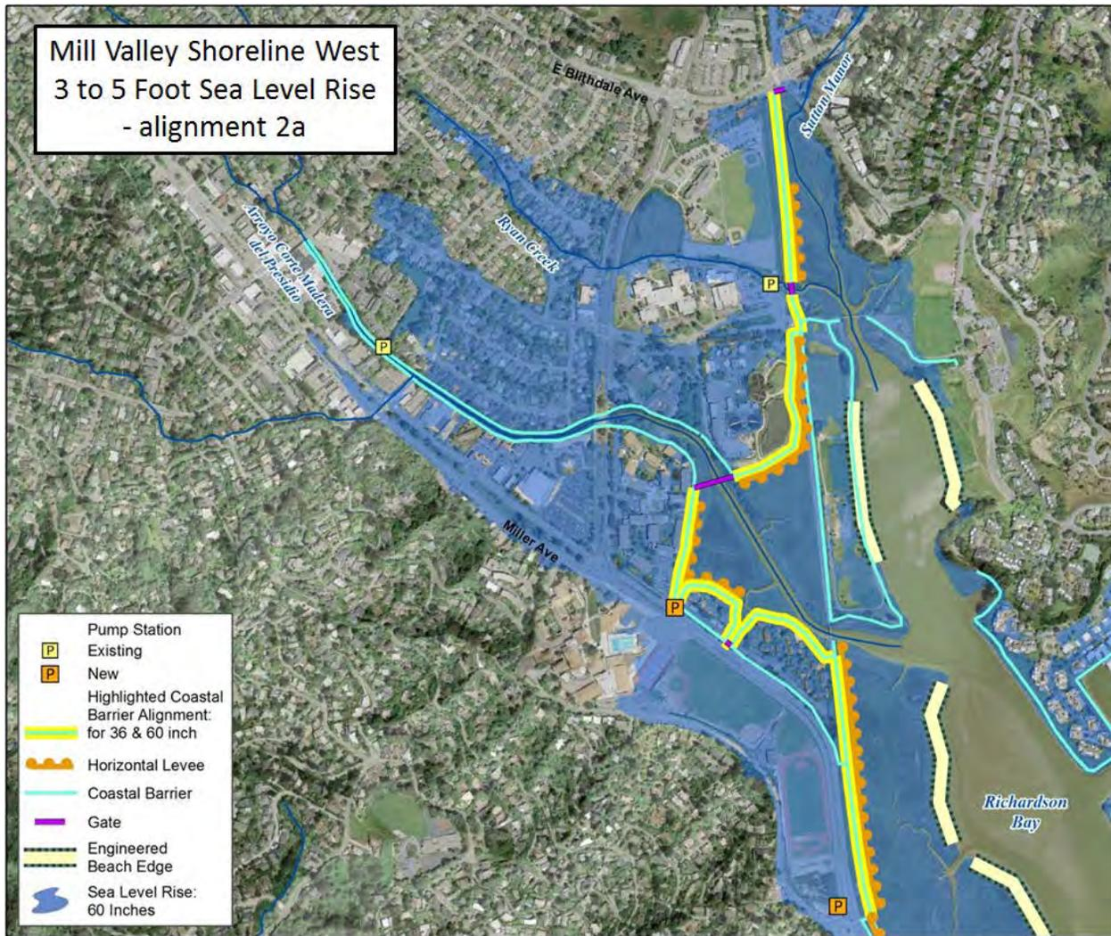
**Figure 47: Reach 3 Alignment 2a. 36 and 60 Inch LDCF Alignment.**
