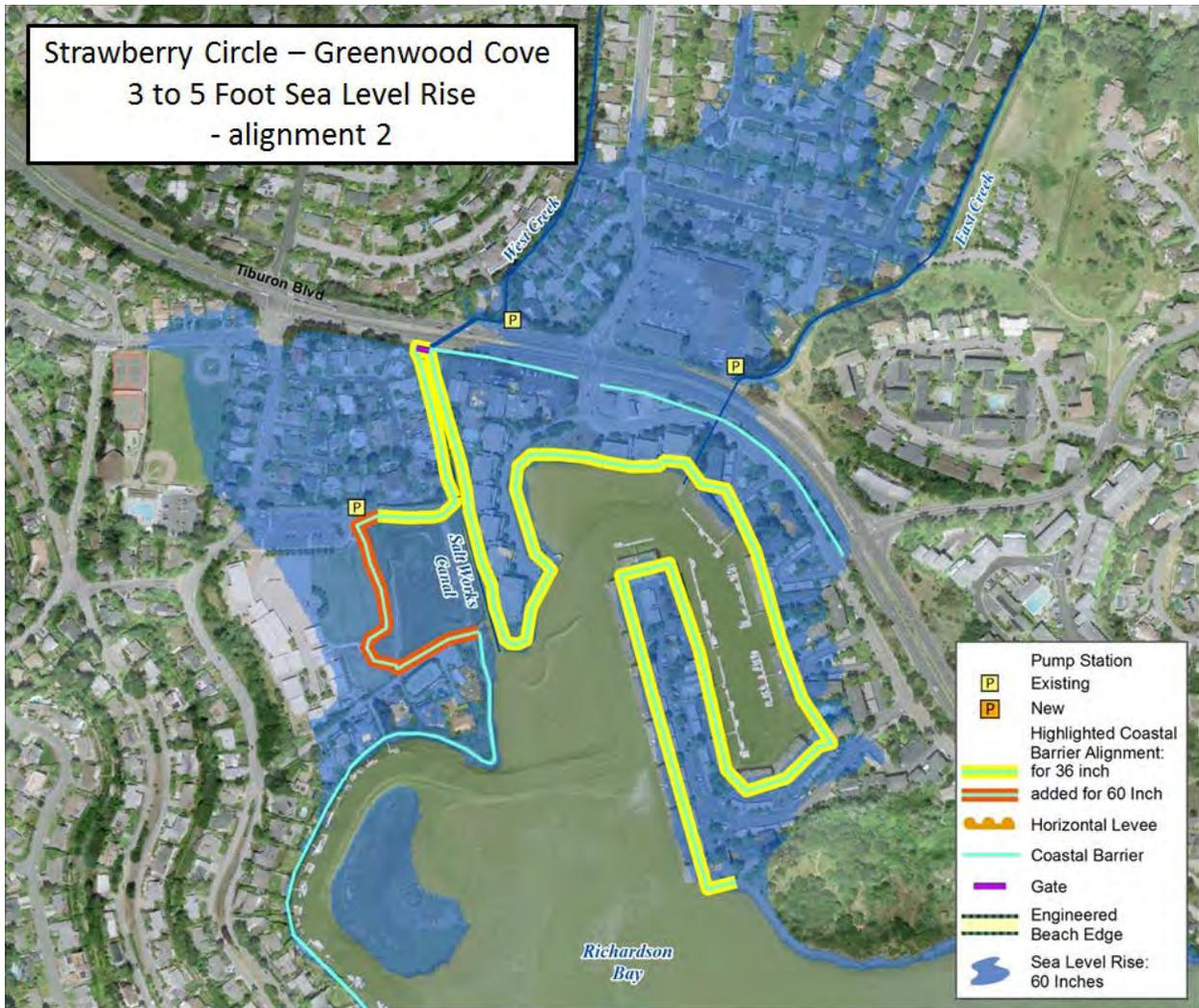
**Figure 56: Reach 7, Alignment 2. 36 and 60 Inch LDCF Alignment.**
