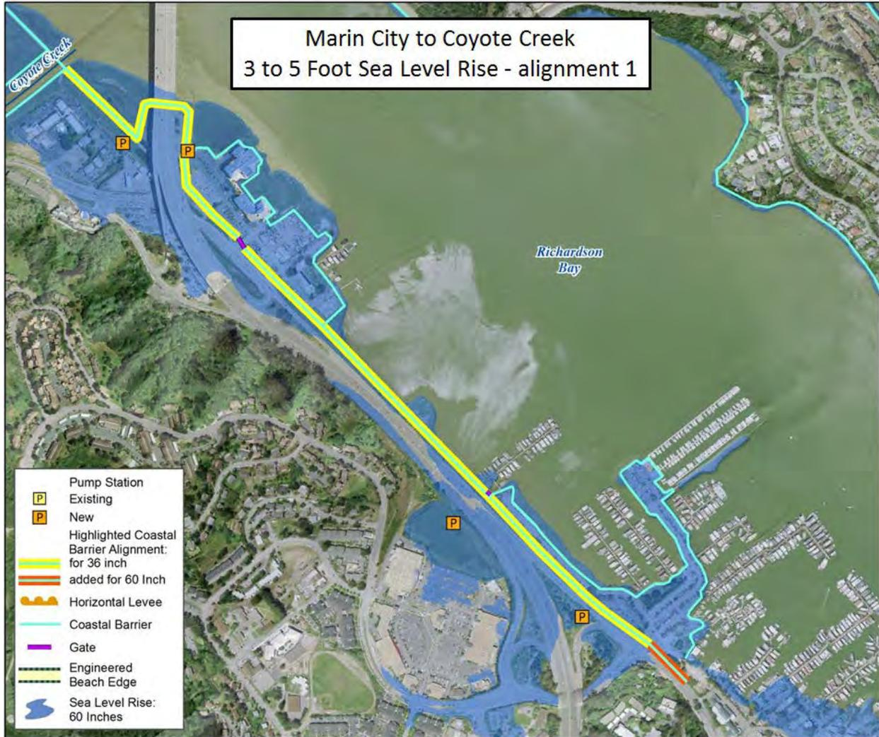
**Figure 40: Reach 1, Alignment 1. 36 and 60 Inch Sea Level Rise LDCF Alignment (60 Inch Sea Level Rise Extensions In Red).**
