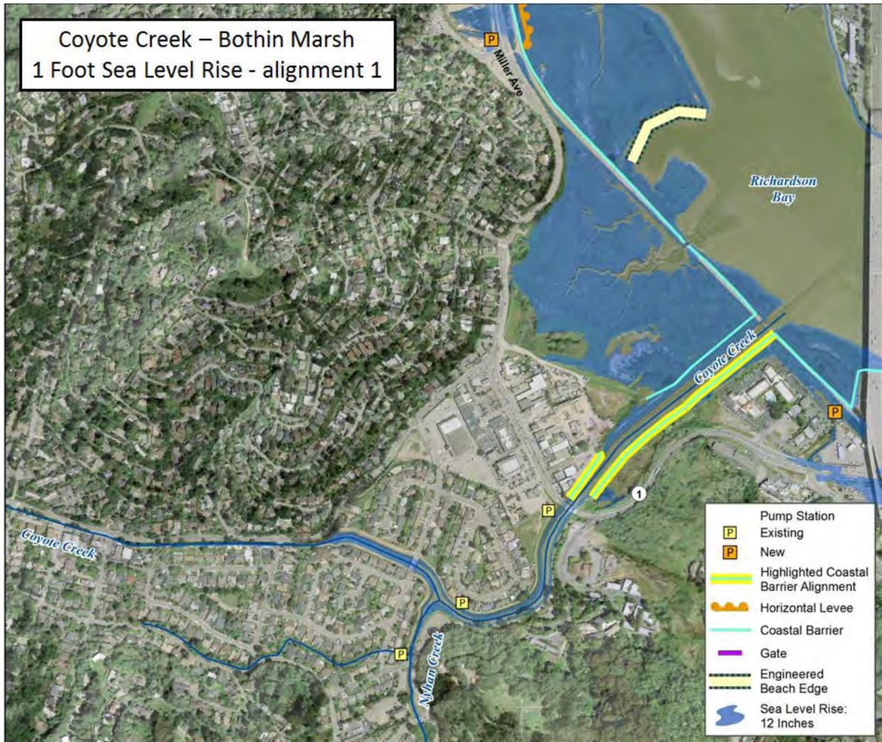
**Figure 32: Reach 2, Alignment 1. Possible Limit of Direct Coastal Flooding Barrier Alignment.**
