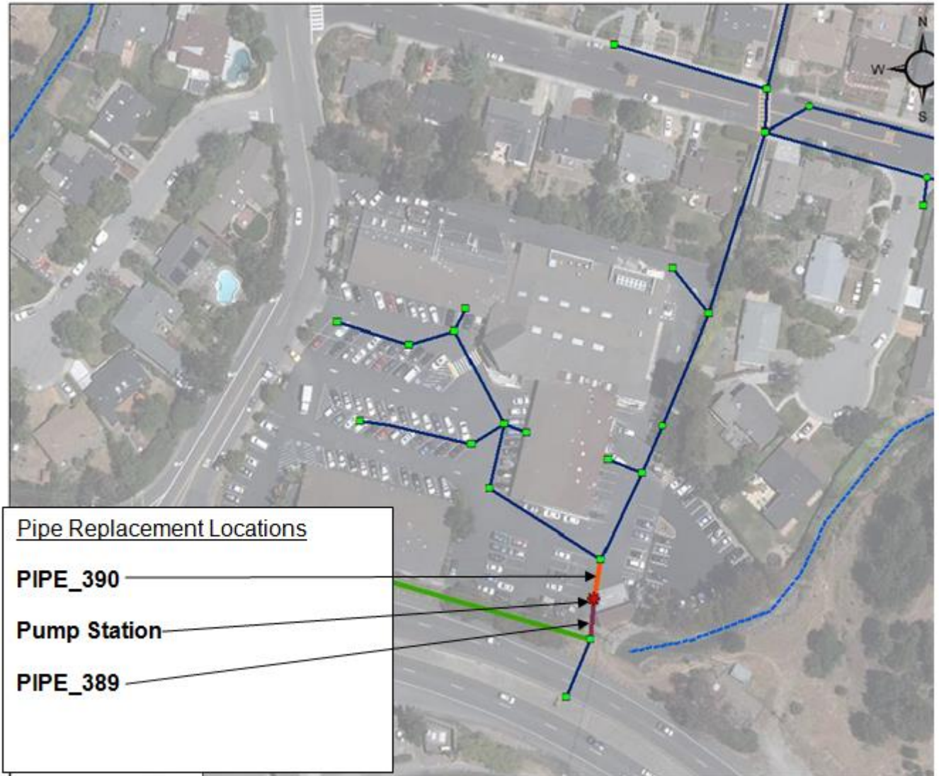
Figure 5-4: Corrugated Metal Pipes Replacements
