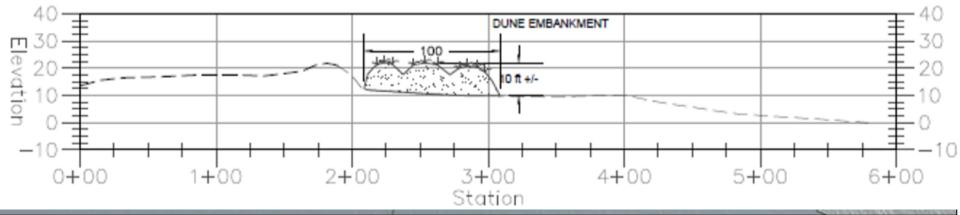
Seadrift East: Alternative 2 more structural versions of nature-based infrastructure, including only a cobble-gravel berm in the Seadrift West and East reaches where there is limited space
