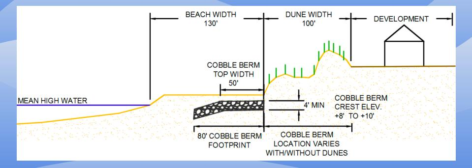
The minimum dune width is 50 feet (foredune and dune embankment features). The minimum top width for cobble berm is 50 feet, while the minimum overall cobble berm footprint is 80 feet including the seaward sloping face. The minimum beach width is 100 feet from either the 50 feet of dunes or the 50 feet of cobble-gravel berm top width.
