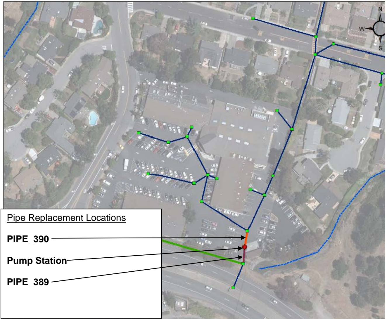
Figure 5-4: Corrugated Metal Pipes Replacements
