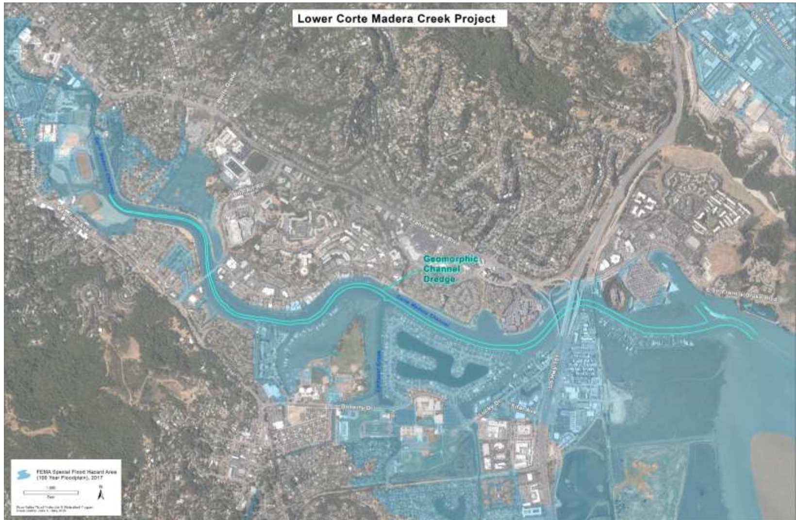
Draft geomorphic dredge concept design for Corte Madera Creek (inner green lines)
